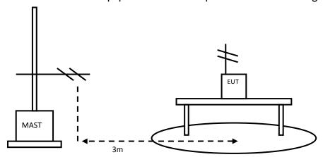
The Equipment Under Test (EUT) was set up on a non-conductive table in the semi-anechoic chamber. The test was performed at the distance of 3 m between the EUT and the receiving antenna. The radiated emissions measurements were made in a typical installation configuration. Then start the test software ES-K1. Sweep the whole frequency band through the range from 30MHz to 1GHz or above, using receive log period antenna HL562 or Ridge horn antenna HF906.
