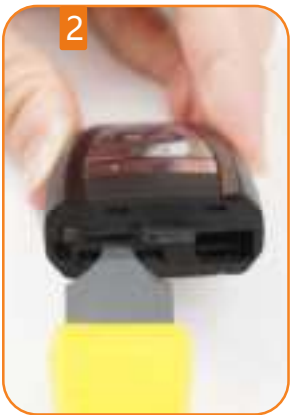
Use the tool into the gap to separate the shell
