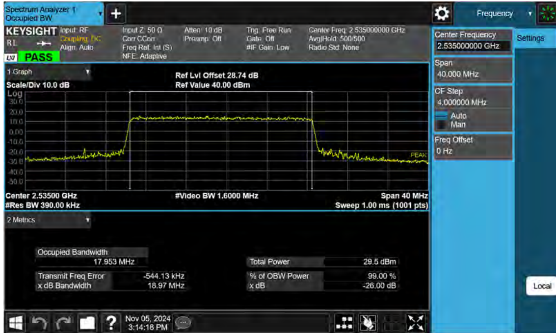
Sub6 n7. Occupied Bandwidth Plot (20 M BW Ch.507000 64QAM)
