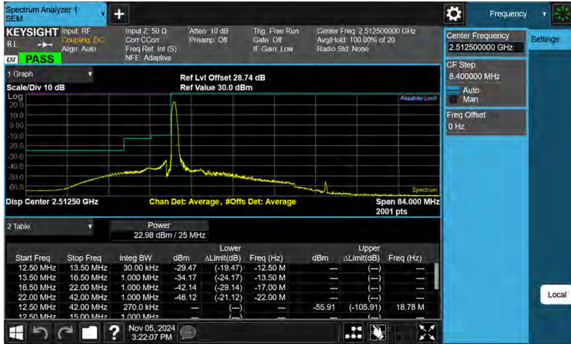
Sub6 n7. Low Channel Edge Plot (25 MHz Ch.502500 BPSK RB 1)-1
