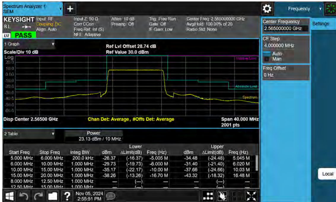
Sub6 n7. High Channel Edge Plot (10 MHz Ch.513000 BPSK)
