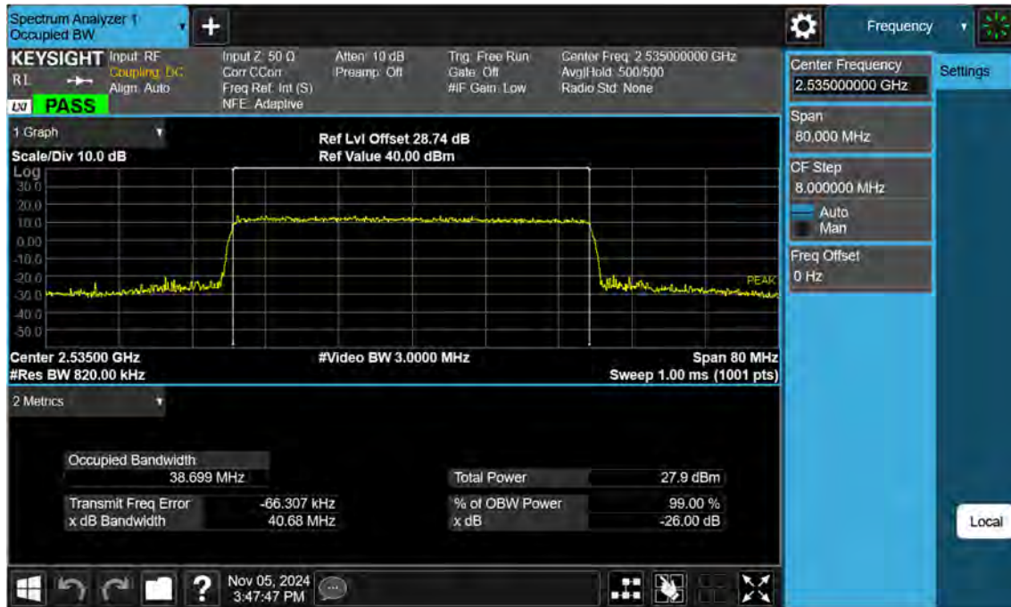
Sub6 n7. Occupied Bandwidth Plot (40 M BW Ch.507000 256QAM)
