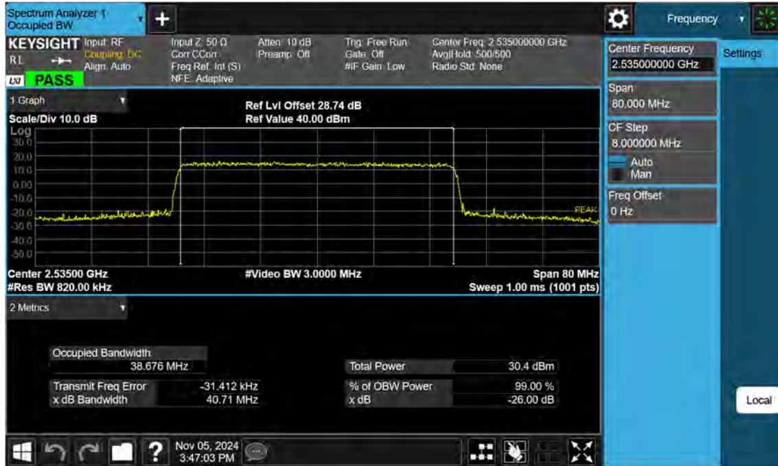
Sub6 n7. Occupied Bandwidth Plot (40 M BW Ch.507000 16QAM)
