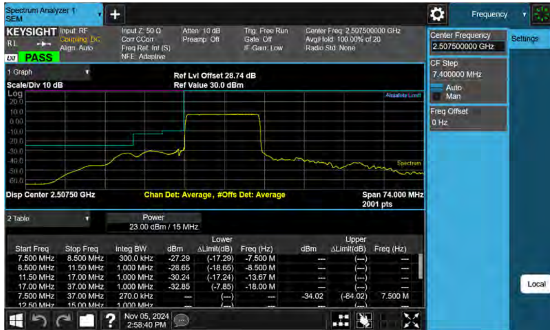
Sub6 n7. Low Channel Edge Plot (15 MHz Ch.501500 BPSK)-1
