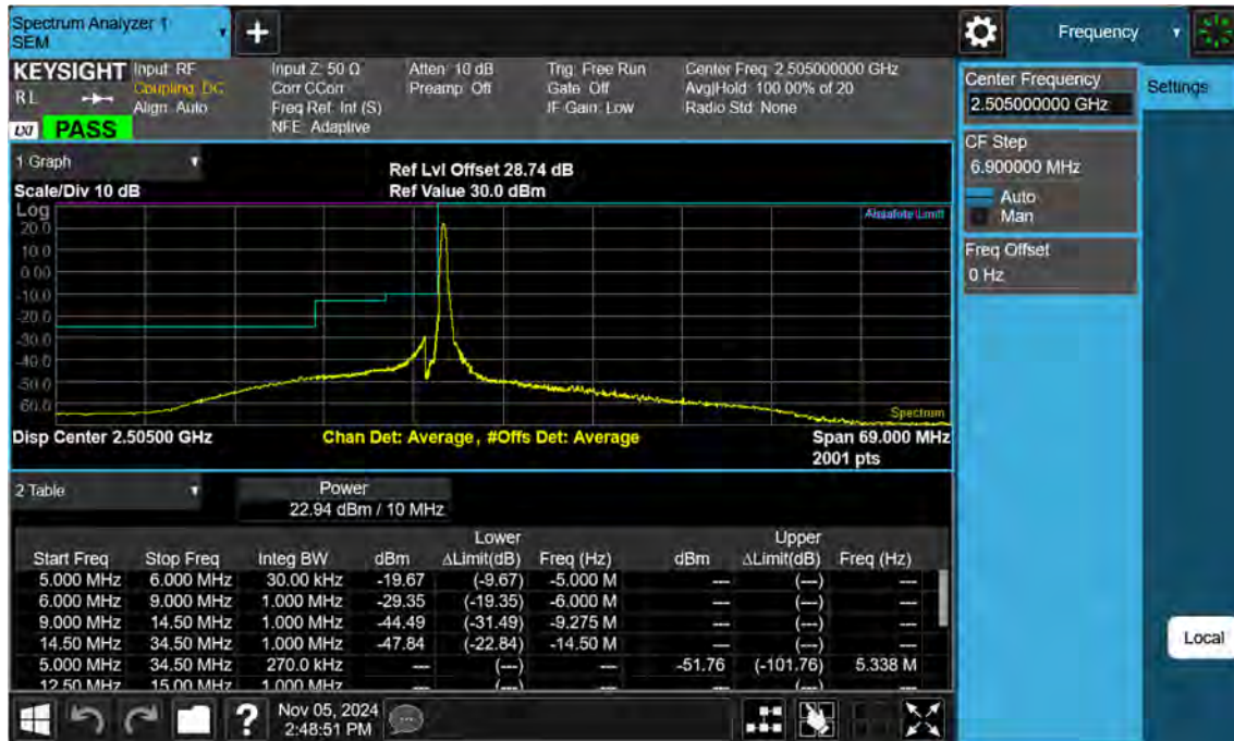
Sub6 n7. Low Channel Edge Plot (10 MHz Ch.501000 BPSK RB 1)-1
