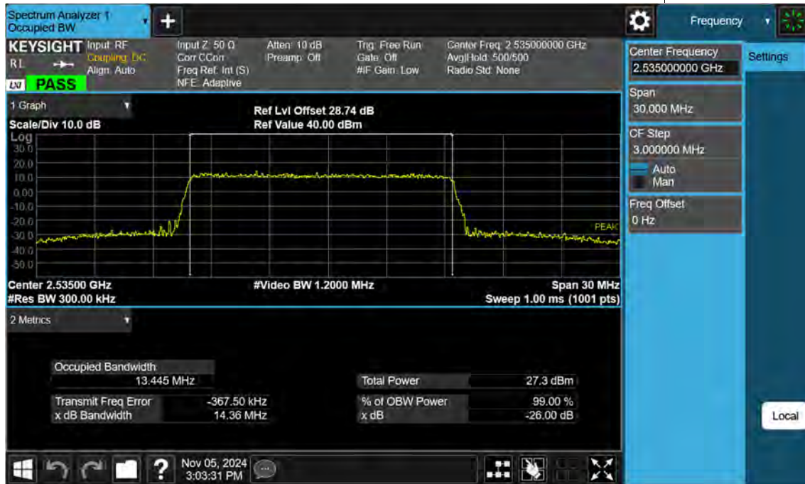
Sub6 n7. Occupied Bandwidth Plot (15 M BW Ch.507000 256QAM)
