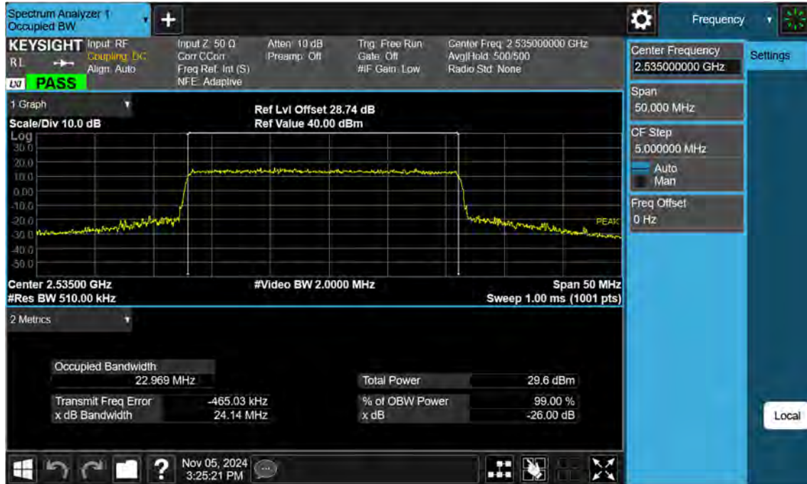
Sub6 n7. Occupied Bandwidth Plot (25 M BW Ch.507000 64QAM)
