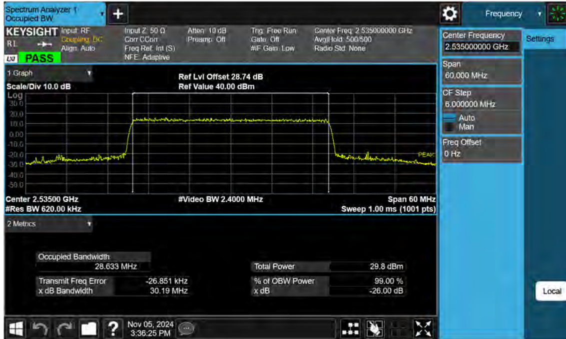
Sub6 n7. Occupied Bandwidth Plot (30 M BW Ch.507000 64QAM)
