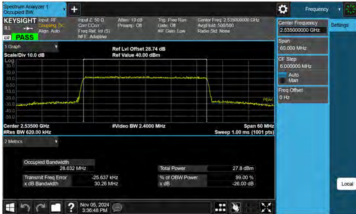
Sub6 n7. Occupied Bandwidth Plot (30 M BW Ch.507000 256QAM)
