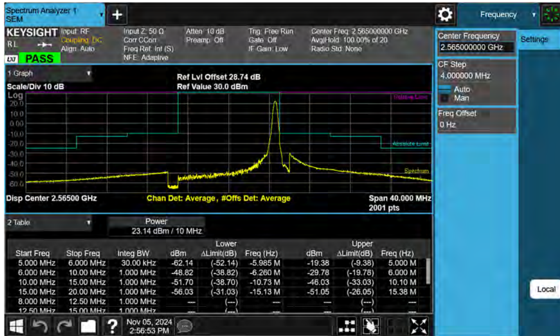
Sub6 n7. High Channel Edge Plot (10 MHz Ch.513000 BPSK RB 1)
