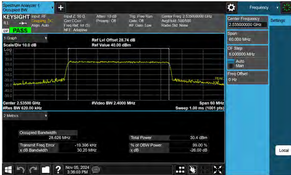
Sub6 n7. Occupied Bandwidth Plot (30 M BW Ch.507000 16QAM)
