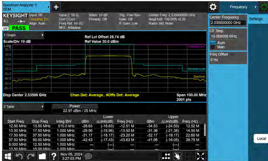
Sub6 n7. Mid Channel Edge Plot (25 MHz Ch.507000 BPSK)
