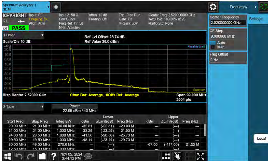
Sub6 n7. Low Channel Edge Plot (40 MHz Ch.504000 BPSK RB 1)-1
