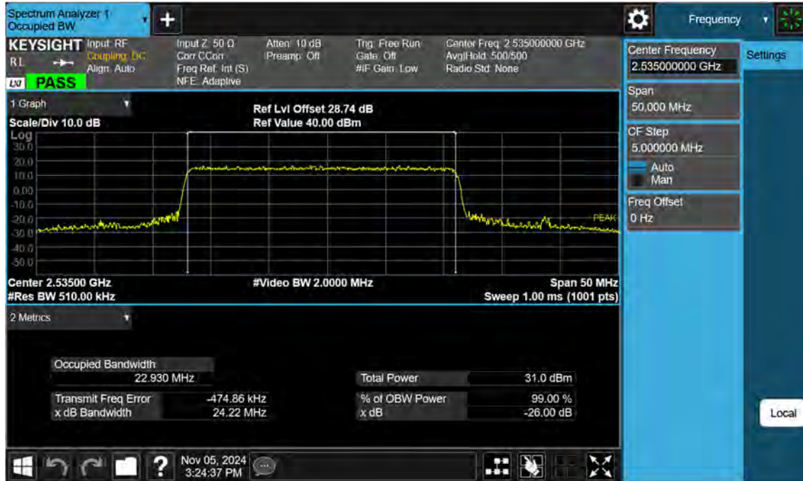
Sub6 n7. Occupied Bandwidth Plot (25 M BW Ch.507000 QPSK)
