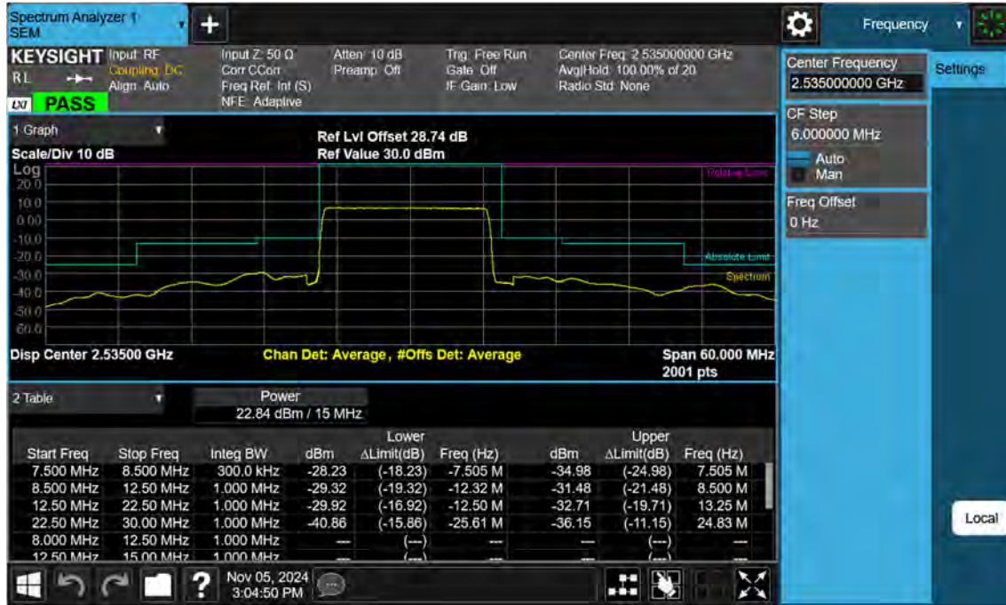
Sub6 n7. Mid Channel Edge Plot (15 MHz Ch.507000 BPSK)
