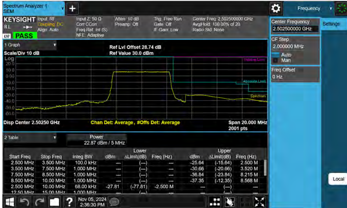
Sub6 n7. Low Channel Edge Plot (5 MHz Ch.500500 BPSK)-2
