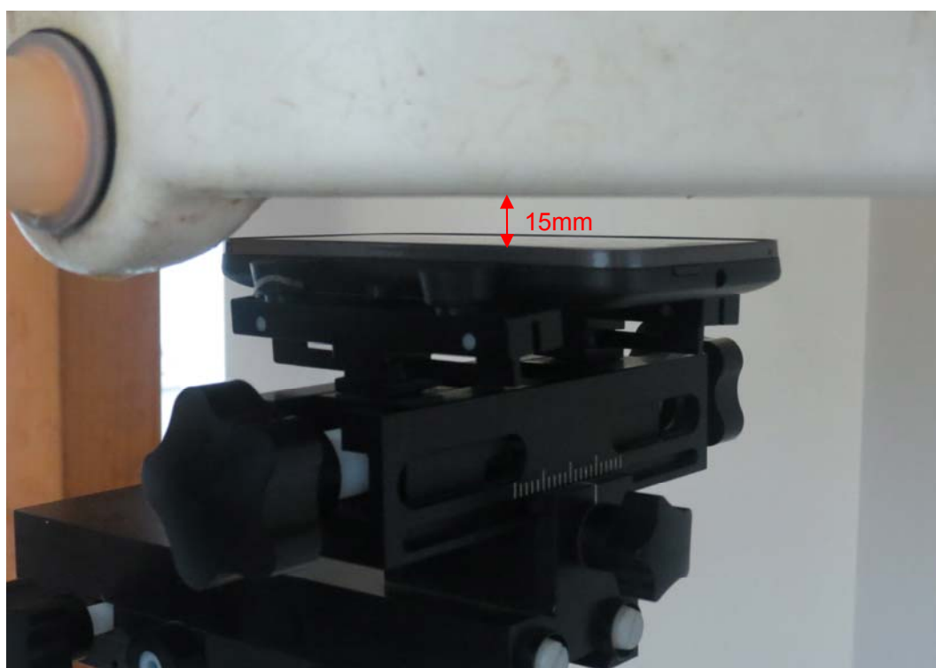
Picture 18: Front Side, the distance from handset to the bottom of the Phantom is 15mm
