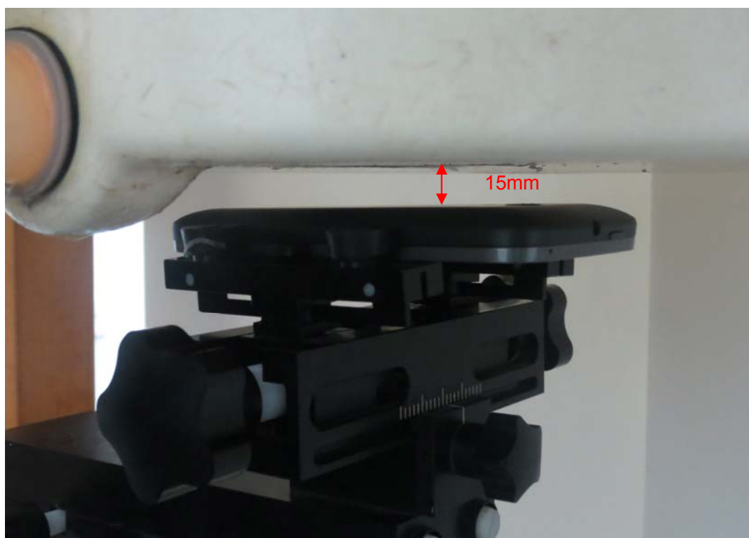
Picture 17: Back Side, the distance from handset to the bottom of the Phantom is 15mm
