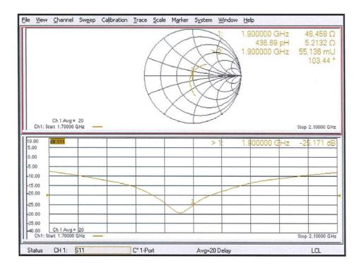
**Calibration for Impedance and Return-loss**
