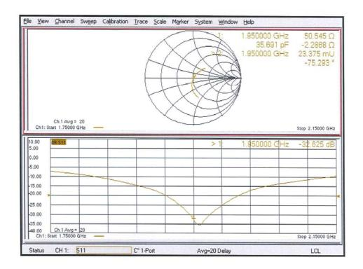
**Calibration for Impedance and Return-loss**
