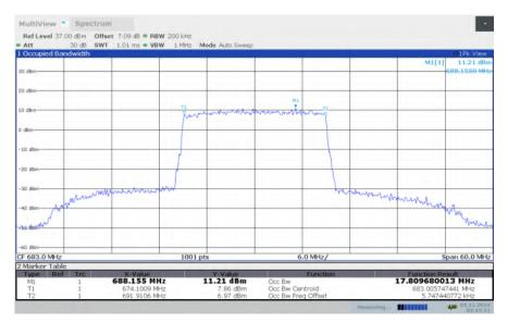
LTE band 71, 20MHz Bandwidth, HIGH, QPSK (99% BW)
