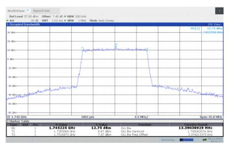
LTE band 66, 15MHz Bandwidth, HIGH, QPSK (99% BW)
