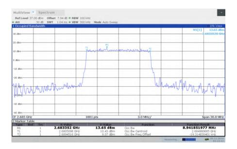
LTE band 41, 10MHz Bandwidth, HIGH, 16QAM (99% BW)
