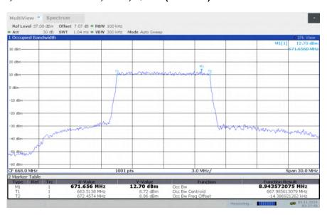
LTE band 71, 10MHz Bandwidth, LOW, 16QAM (99% BW)
