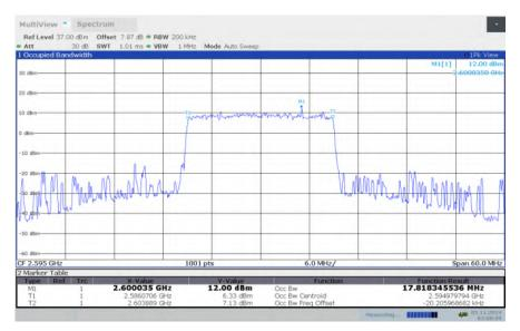
LTE band 38, 20MHz Bandwidth, HIGH, QPSK (99% BW)
