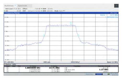
LTE band 2, 1.4MHz Bandwidth, MID, 16QAM (-26dBc BW)
