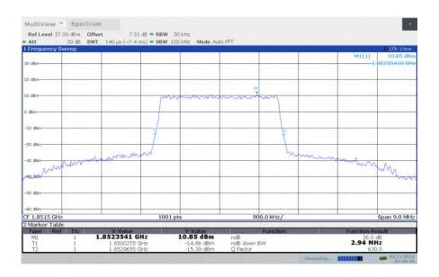
LTE band 2, 3MHz Bandwidth, MID, QPSK (-26dBc BW)
