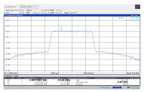
LTE band 2, 3MHz Bandwidth, HIGH, 64QAM (-26dBc BW)
