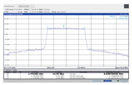
LTE band 66, 10MHz Bandwidth, HIGH, 64QAM (99% BW)
