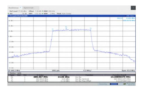
LTE band 71, 15MHz Bandwidth, HIGH, 16QAM (99% BW)
