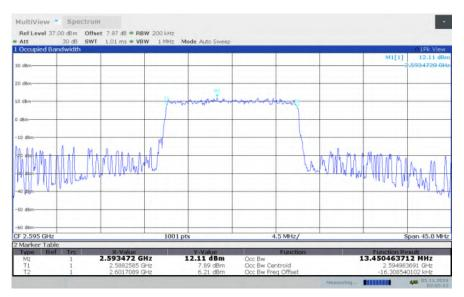
LTE band 38, 15MHz Bandwidth, HIGH, QPSK (99% BW)
