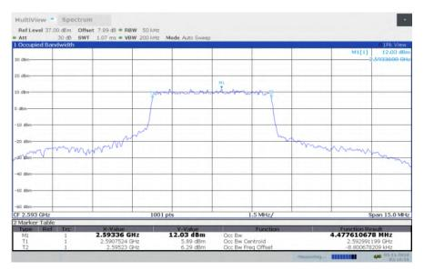
LTE band 41, 5MHz Bandwidth, HIGH, QPSK (99% BW)
