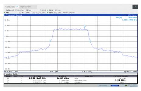
LTE band 2, 1.4MHz Bandwidth, LOW, 16QAM (-26dBc BW)
