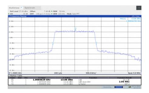
LTE band 2, 3MHz Bandwidth, HIGH, 16QAM (-26dBc BW)
