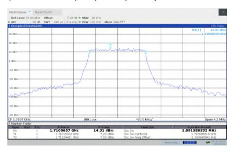
LTE band 66, 1.4MHz Bandwidth, LOW, 64QAM (99% BW)
