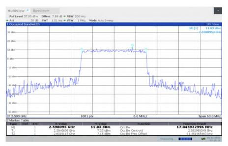
LTE band 41, 20MHz Bandwidth, HIGH, QPSK (99% BW)
