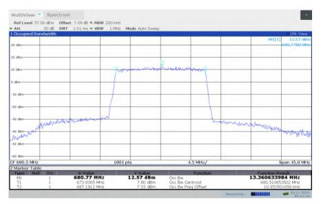
LTE band 71, 15MHz Bandwidth, HIGH, QPSK (99% BW)
