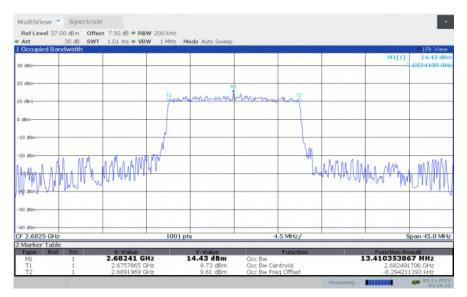
LTE band 41, 15MHz Bandwidth, HIGH, 64QAM (99% BW)
