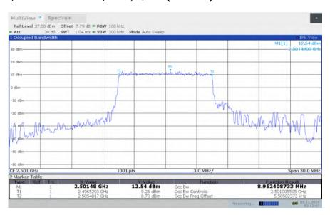
LTE band 41, 10MHz Bandwidth, LOW, 16QAM (99% BW)
