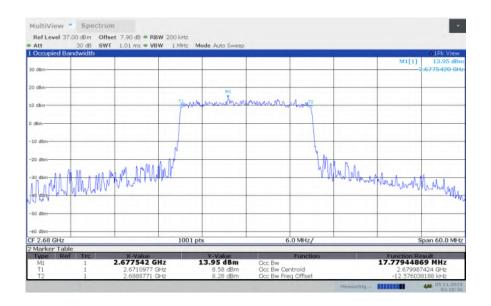
LTE band 41, 20MHz Bandwidth, HIGH, 16QAM (99% BW)
