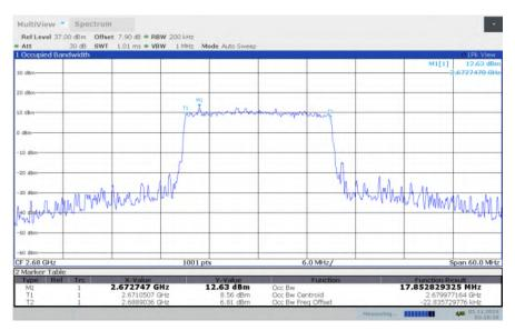
LTE band 41, 20MHz Bandwidth, HIGH, 64QAM (99% BW)
