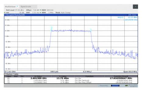
LTE band 38, 20MHz Bandwidth, HIGH, 64QAM (99% BW)
