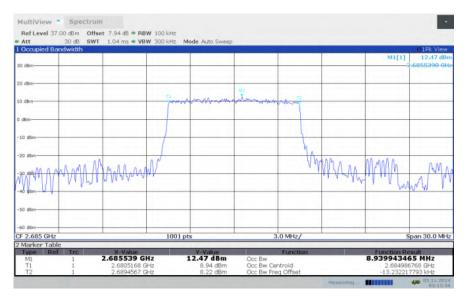
LTE band 41, 10MHz Bandwidth, HIGH, 64QAM (99% BW)
