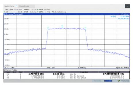
LTE band 66, 20MHz Bandwidth, HIGH, 64QAM (99% BW)
