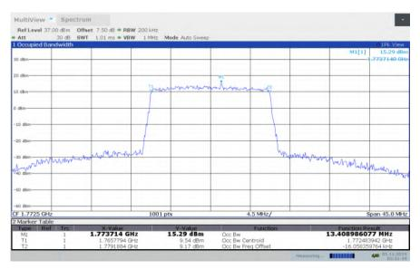
LTE band 66, 15MHz Bandwidth, HIGH, 64QAM (99% BW)
