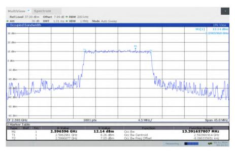
LTE band 41, 15MHz Bandwidth, HIGH, QPSK (99% BW)
