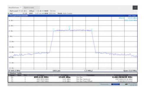
LTE band 71, 5MHz Bandwidth, HIGH, 16QAM (99% BW)
