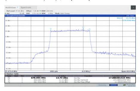
LTE band 71, 20MHz Bandwidth, LOW, 16QAM (99% BW)
