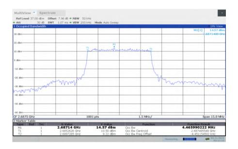
LTE band 41, 5MHz Bandwidth, HIGH, 16QAM (99% BW)
