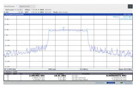
LTE band 41, 10MHz Bandwidth, HIGH, QPSK (99% BW)
