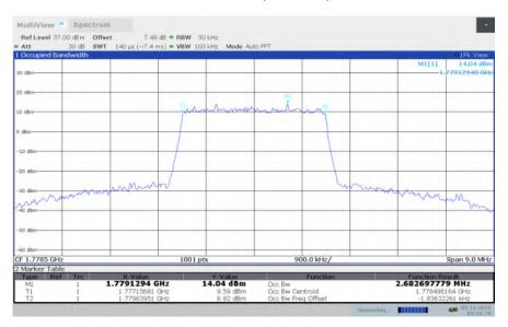
LTE band 66, 3MHz Bandwidth, HIGH, 64QAM (99% BW)
