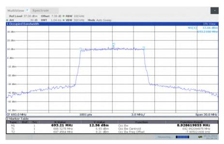
LTE band 71, 10MHz Bandwidth, HIGH, 64QAM (99% BW)
