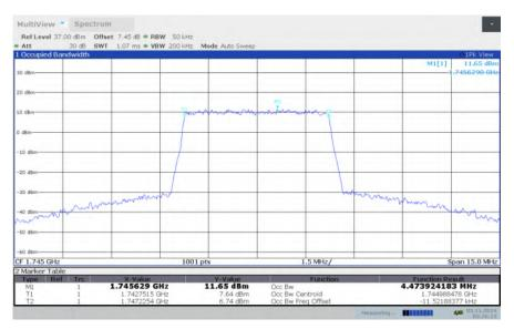
LTE band 66, 5MHz Bandwidth, HIGH, QPSK (99% BW)
