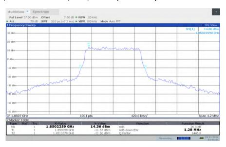
LTE band 2, 1.4MHz Bandwidth, LOW, 64QAM (-26dBc BW)
