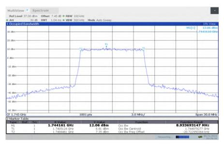
LTE band 66, 10MHz Bandwidth, HIGH, QPSK (99% BW)
