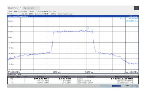
LTE band 71, 20MHz Bandwidth, HIGH, 16QAM (99% BW)
