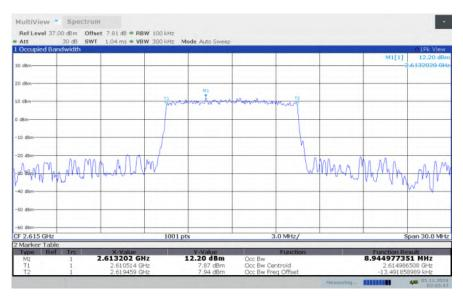
LTE band 38, 10MHz Bandwidth, HIGH, 64QAM (99% BW)
