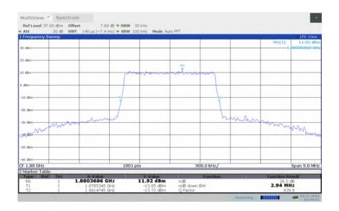
LTE band 2, 3MHz Bandwidth, MID, 64QAM (-26dBc BW)
