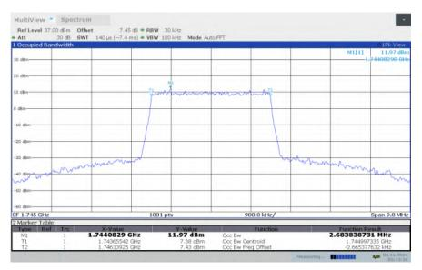
LTE band 66, 3MHz Bandwidth, HIGH, QPSK (99% BW)
