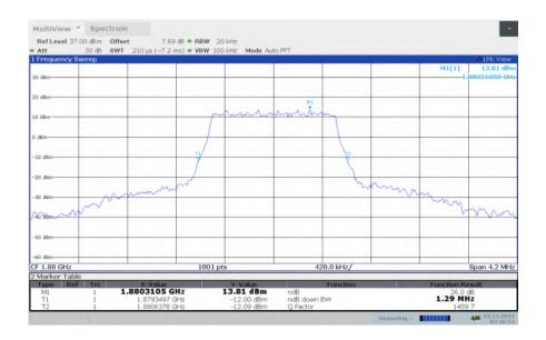
LTE band 2, 1.4MHz Bandwidth, MID, 64QAM (-26dBc BW)
