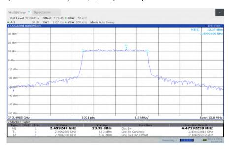
LTE band 41, 5MHz Bandwidth, LOW, 16QAM (99% BW)
