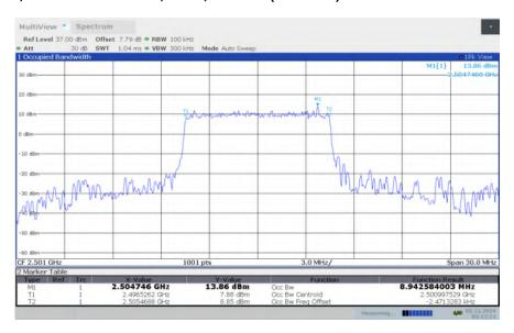
LTE band 41, 10MHz Bandwidth, LOW, 64QAM (99% BW)
