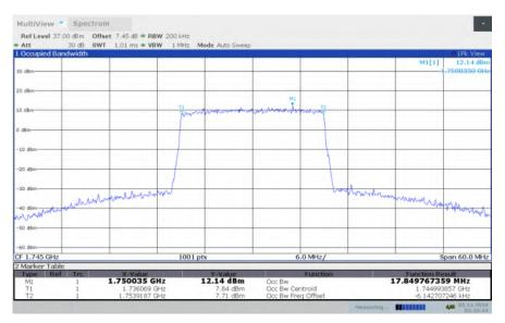
LTE band 66, 20MHz Bandwidth, HIGH, QPSK (99% BW)
