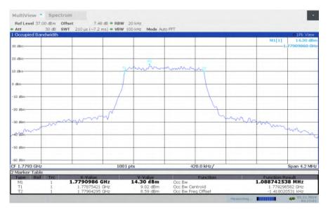
LTE band 66, 1.4MHz Bandwidth, HIGH, 64QAM (99% BW)
