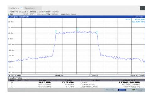
LTE band 71, 10MHz Bandwidth, HIGH, 16QAM (99% BW)
