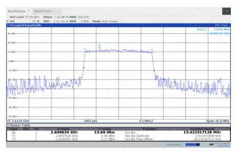
LTE band 38, 15MHz Bandwidth, HIGH, 64QAM (99% BW)
