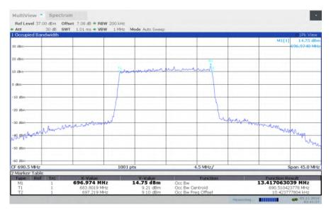
LTE band 71, 15MHz Bandwidth, HIGH, 64QAM (99% BW)
