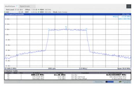
LTE band 71, 10MHz Bandwidth, HIGH, QPSK (99% BW)
