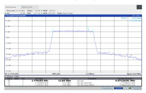
LTE band 66, 5MHz Bandwidth, HIGH, 64QAM (99% BW)
