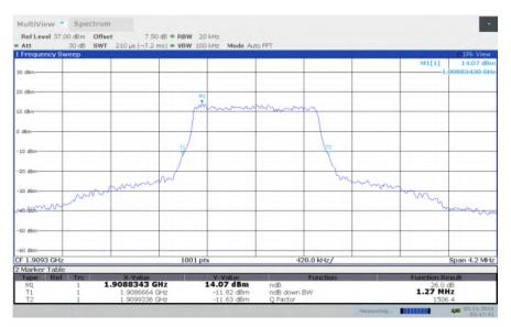
LTE band 2, 1.4MHz Bandwidth, HIGH, 64QAM (-26dBc BW)
