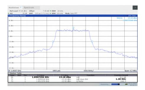
LTE band 2, 1.4MHz Bandwidth, MID, QPSK (-26dBc BW)
