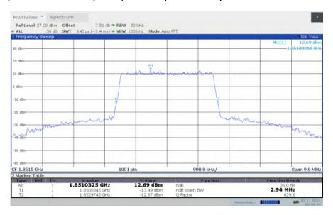
LTE band 2, 3MHz Bandwidth, LOW, 64QAM (-26dBc BW)
