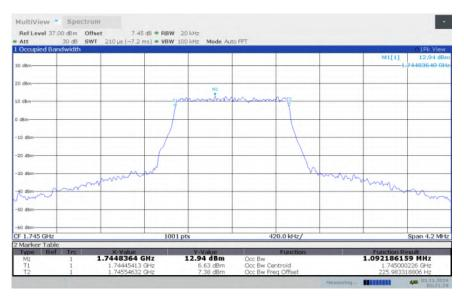
LTE band 66, 1.4MHz Bandwidth, HIGH, QPSK (99% BW)
