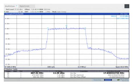
LTE band 71, 20MHz Bandwidth, HIGH, 64QAM (99% BW)
