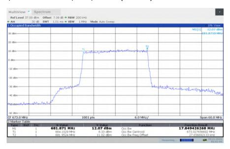
LTE band 71, 20MHz Bandwidth, LOW, 64QAM (99% BW)
