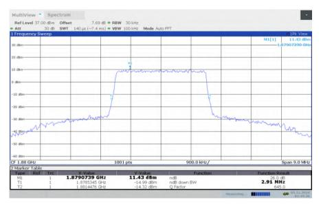
LTE band 2, 3MHz Bandwidth, HIGH, QPSK (-26dBc BW)
