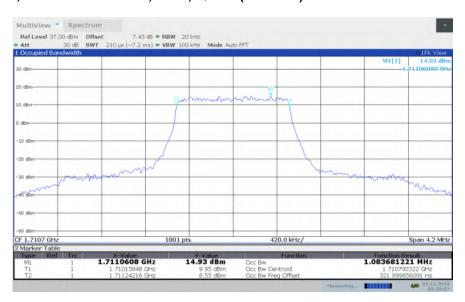
LTE band 66, 1.4MHz Bandwidth, LOW, 16QAM (99% BW)
