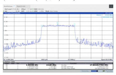
LTE band 41, 20MHz Bandwidth, LOW, 16QAM (99% BW)
