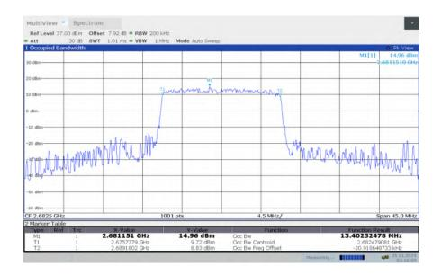
LTE band 41, 15MHz Bandwidth, HIGH, 16QAM (99% BW)
