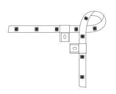
**Trimming the Strip:** The strip can be cut to a desired length at the designated marks. **Make sure the power adapter is unplugged before cutting.**
