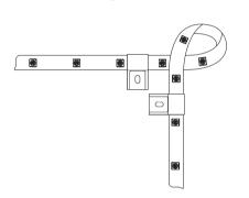
**Trimming the Strip:** The strip can be cut to a desired length at the designated marks. Make sure the power adapter is unplugged before
