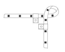
**Trimming the Strip:** The strip can be cut to a desired length at the designated marks. Make sure the power adapter is unplugged before
