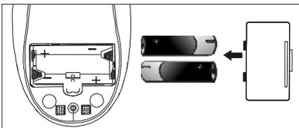
1. Remove the battery compartment cover on the bottom of the mouse.
