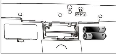
1. Remove the battery compartment cover on the bottom of the cordless keyboard.
