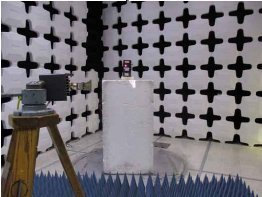
Test Setup for Radiated Emissions, Transmitters– Above 18GHz, Horizontal Polarization
