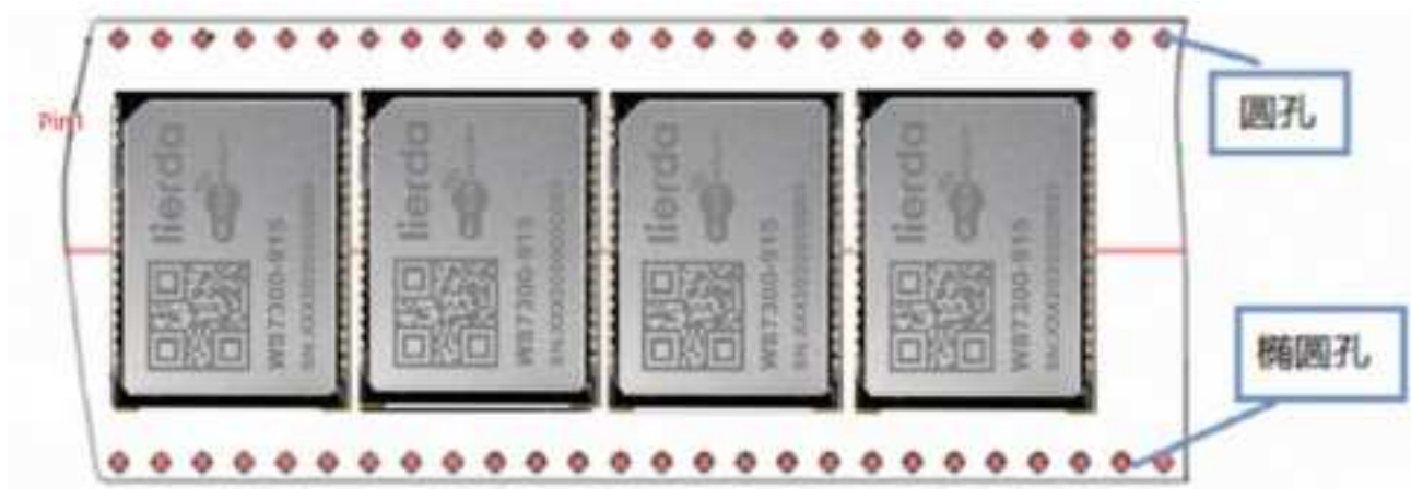
Figure 4 . 3 Schematic diagram of product placement direction
