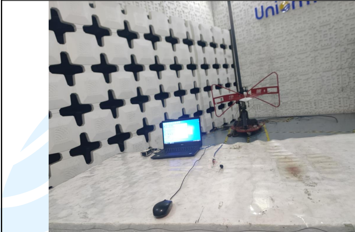
Radiated emission Test Setup (30 MHz~1 GHz)
