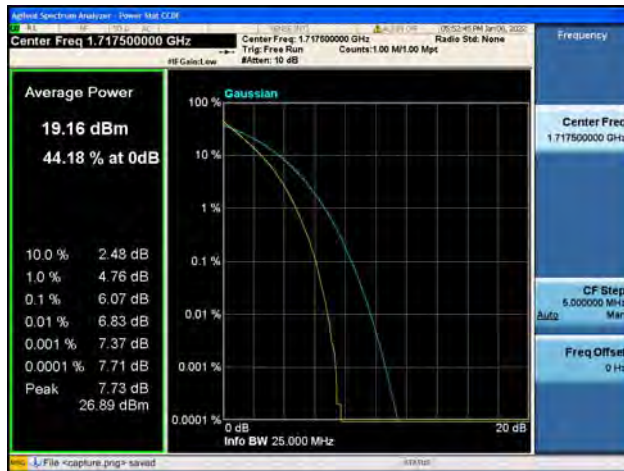
Band66 / 15MHz / Low CH / 64QAM
