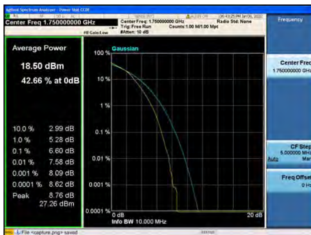
Band4 / 10MHz / High CH / 16QAM
