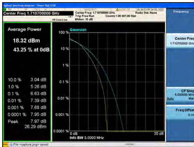
Band4 / 1.4MHz / Mid CH / 16QAM
