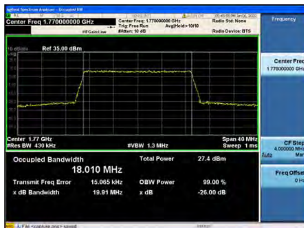
Band66 / 20MHz / High CH / 16QAM
