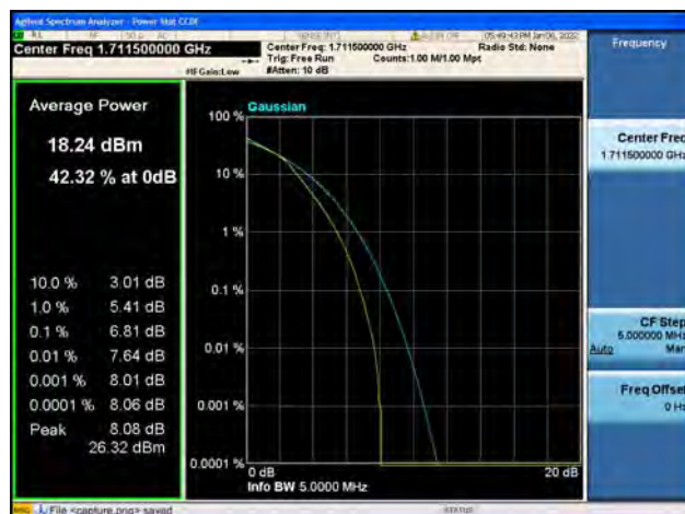
Band66 / 3MHz / Low CH / 16QAM
