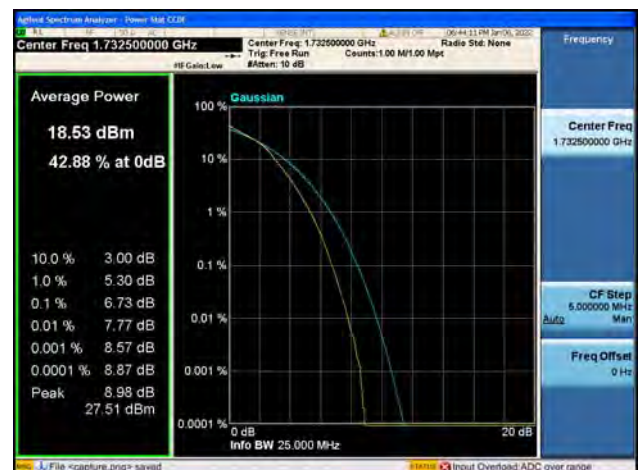
Band4 / 15MHz / Mid CH / 64QAM
