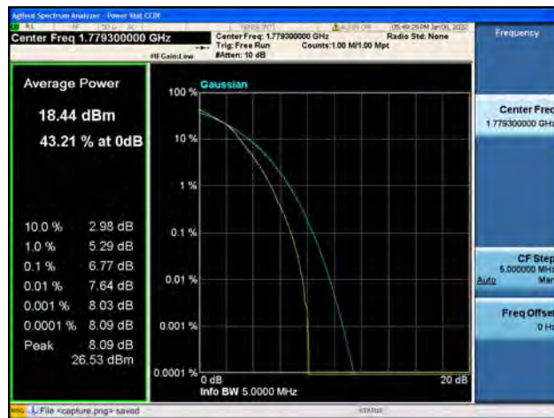
Band66 / 3MHz / Low CH / 16QAM
