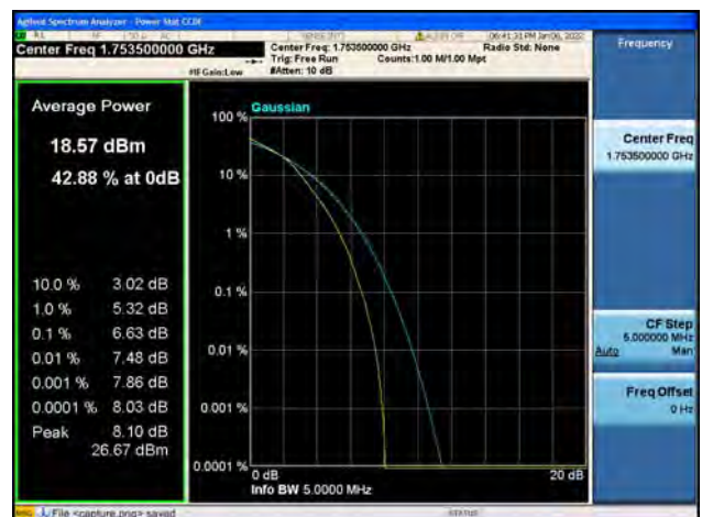
Band4 / 3MHz / High CH / 64QAM
