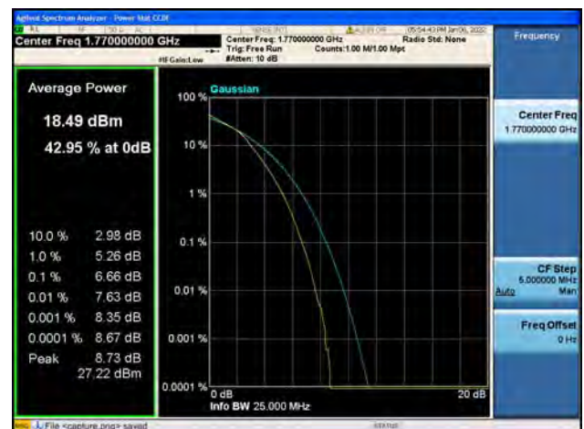
Band66 / 20MHz / High CH / 64QAM
