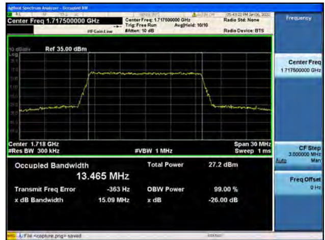
Band66 / 15MHz / Mid CH / QPSK
