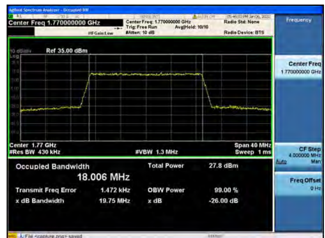
Band66 / 20MHz / High CH / 64QAM
