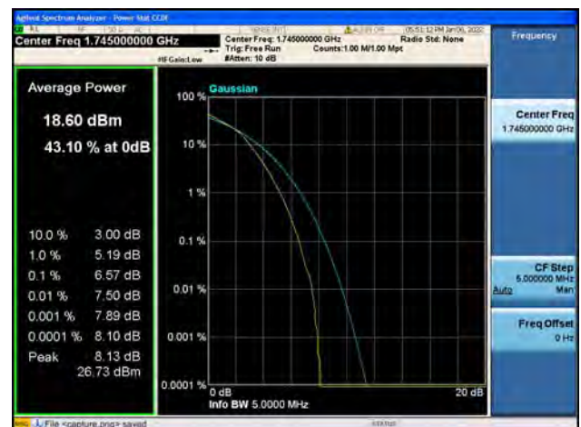
Band66 / 5MHz / Mid CH / 64QAM
