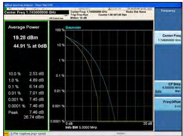
Band66 / 1.4MHz / Mid CH / 64QAM
