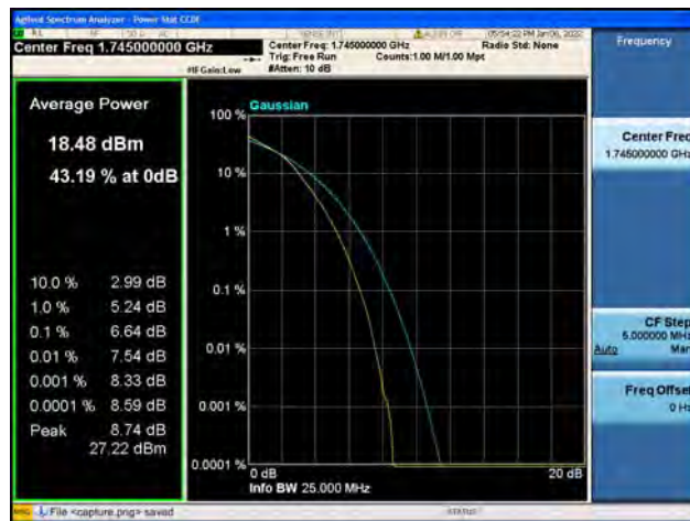
Band66 / 20MHz / High CH / 16QAM
