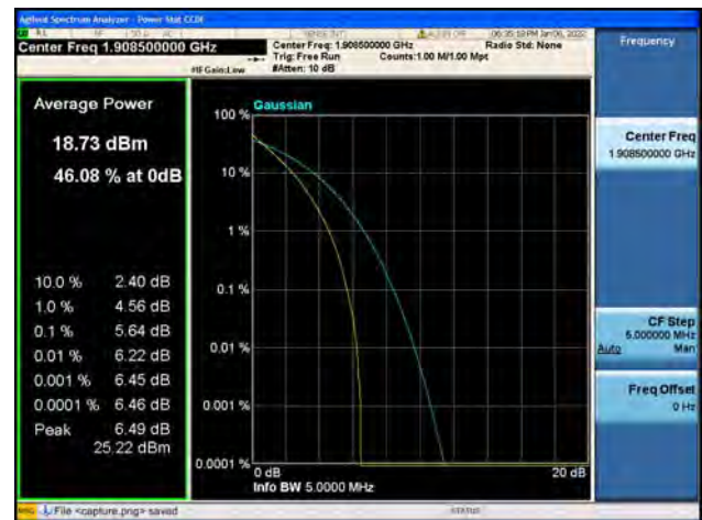
Band2 / 3MHz / High CH / 64QAM
