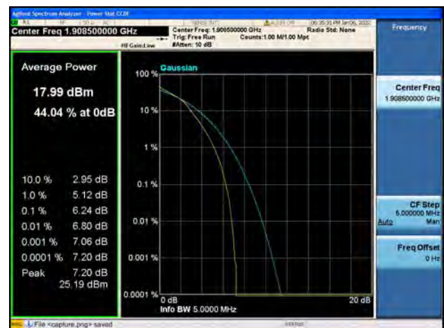
Band2 / 3MHz / High CH / 64QAM
