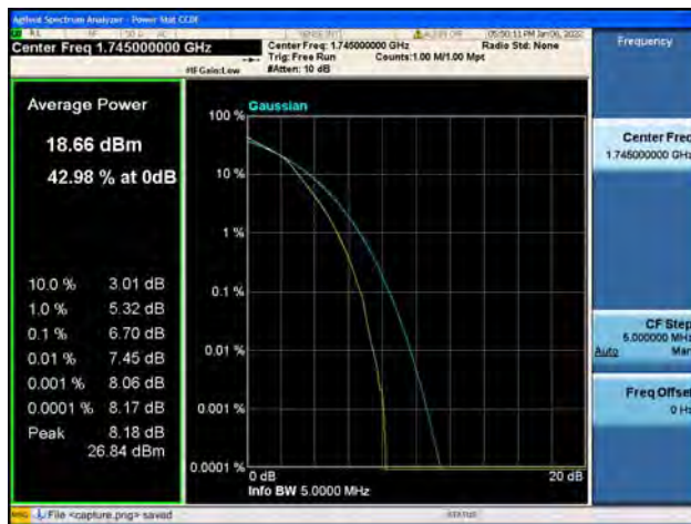
Band66 / 3MHz / High CH / 16QAM
