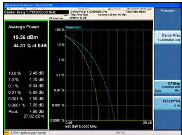
Band4 / 5MHz / Mid CH / 64QAM
