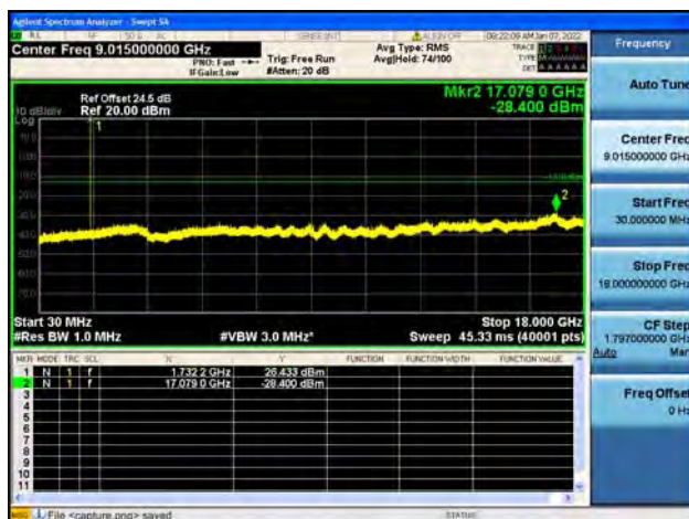
Band4 / 1.4MHz / Mid CH / 16QAM
