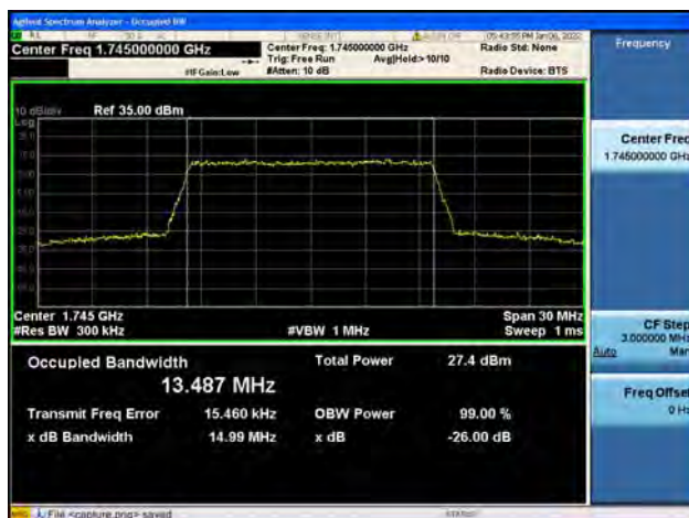
Band66 / 15MHz / Mid CH / 16QAM
