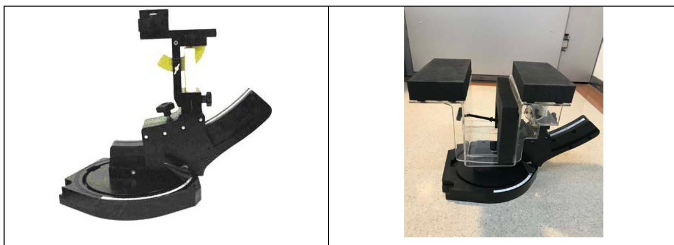
Device holder supplied by SPEAG
