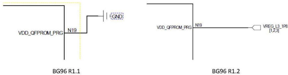
Figure 1: Schematic Designs of BG96 R1.1 and R1.2
