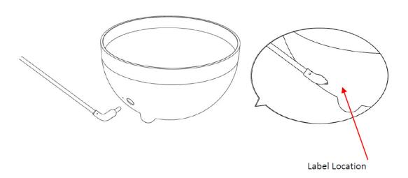
The label shown shall be permanently affixed at a conspicuous location on the device and be readily visible to the user at the time purchase (Labeling requirements per 2.925)
