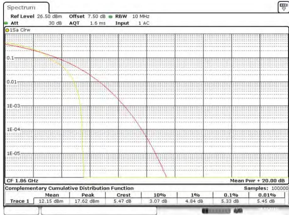
**20.0 MHz PAR – Middle Channel (16QAM, 1RB Size)**
