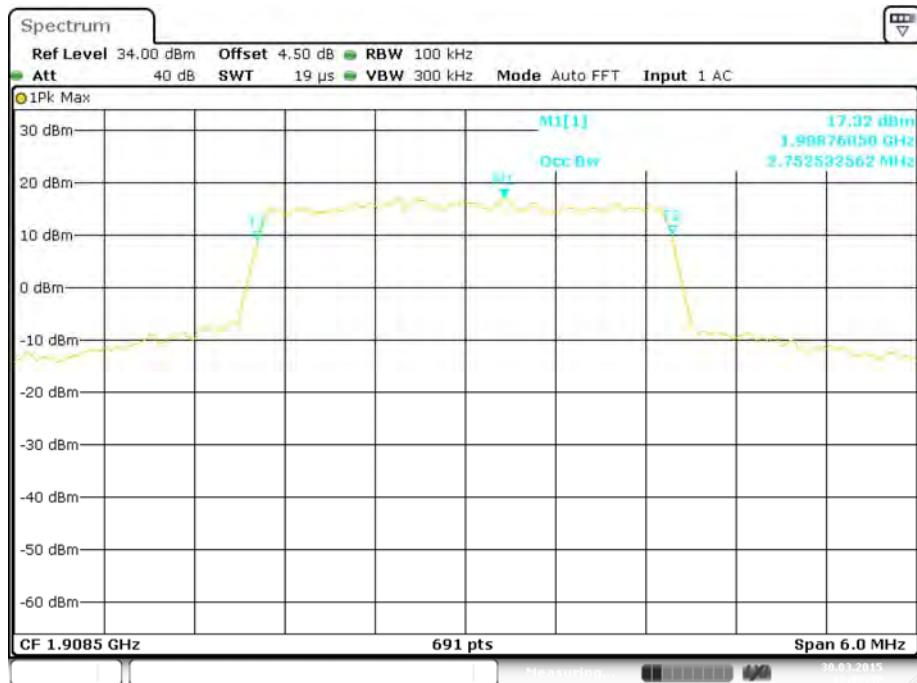
**16-QAM (3.0 MHz) - 99% Occupied Bandwidth, Low channel**
