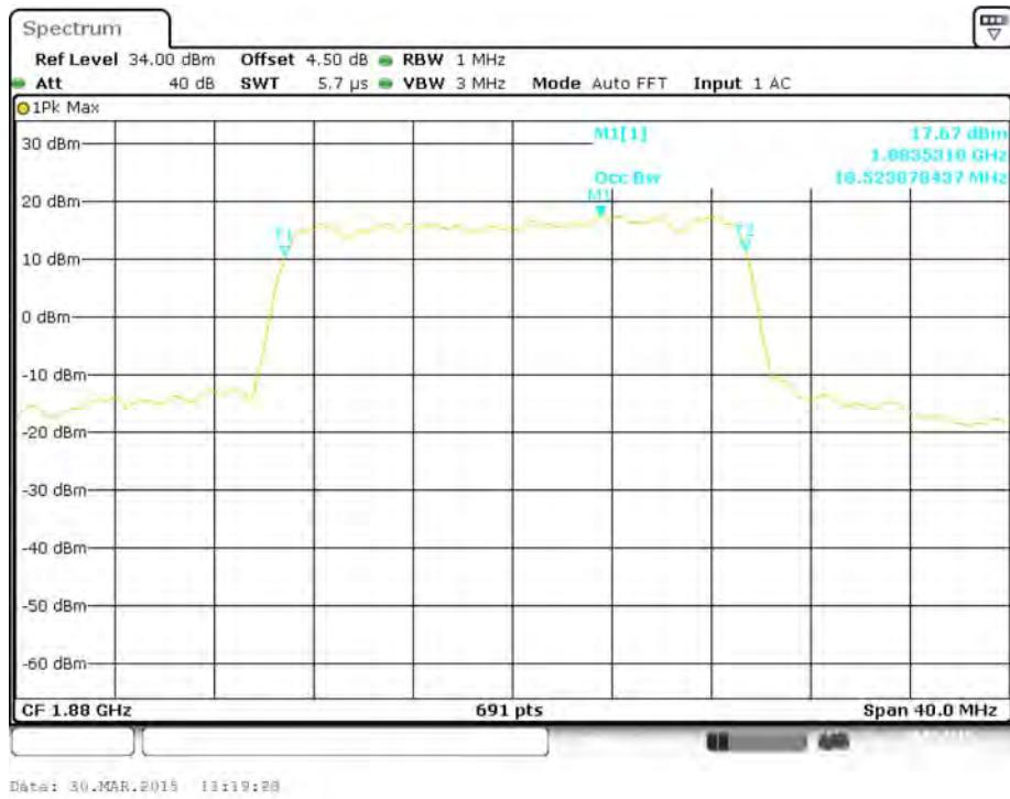
**16-QAM (20.0 MHz) - 99% Occupied Bandwidth, High channel**
