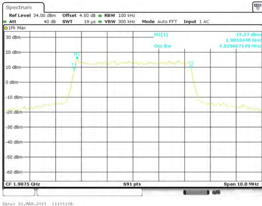
**16-QAM (5.0 MHz) - 99% Occupied Bandwidth, Low channel**
