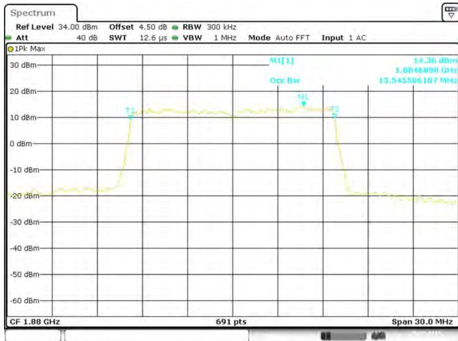
**16-QAM (15.0 MHz) - 99% Occupied Bandwidth, High channel**
