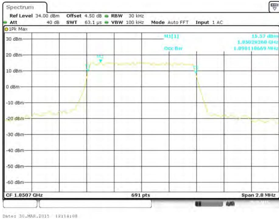
**QPSK (1.4 MHz) - 99% Occupied Bandwidth, Middle channel**
