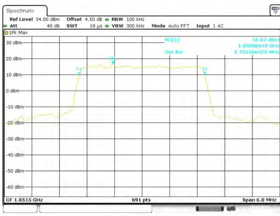
**16-QAM (3.0 MHz) - 99% Occupied Bandwidth, Middle channel**
