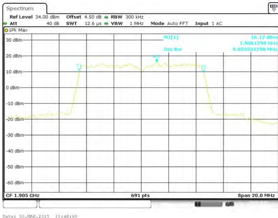
**QPSK (15.0 MHz) - 99% Occupied Bandwidth, Low channel**
