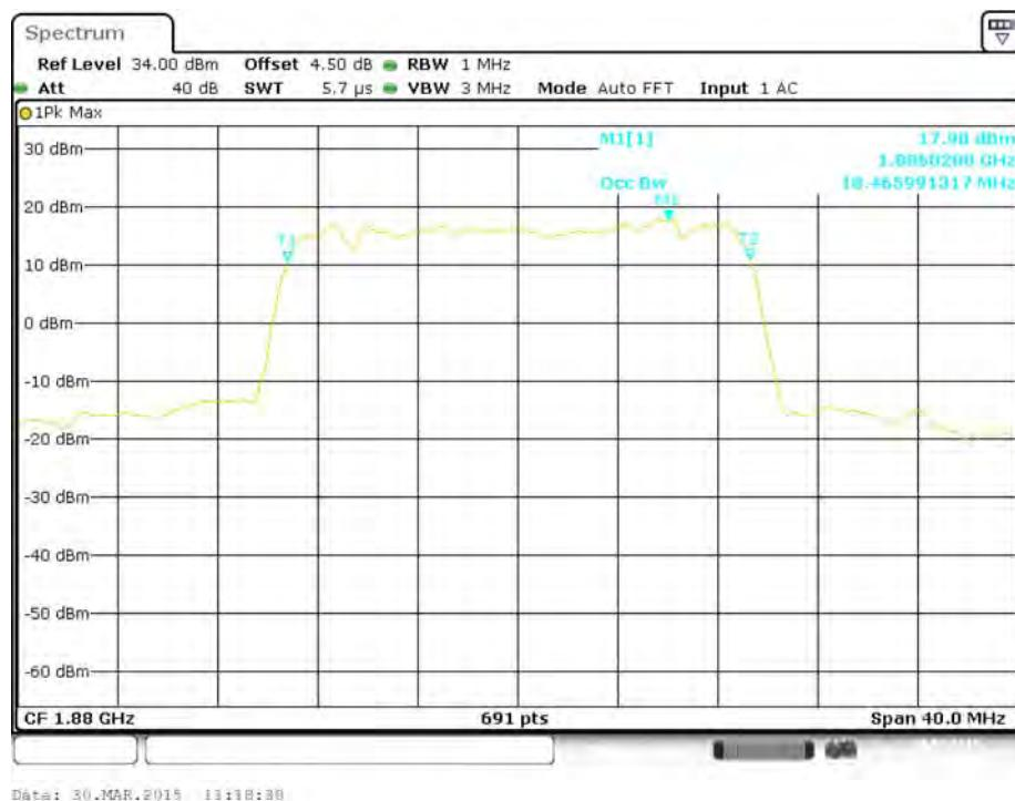
**QPSK (20.0 MHz) - 99% Occupied Bandwidth, High channel**
