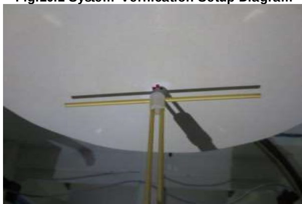
Fig.10.2 Photo of Dipole setup
