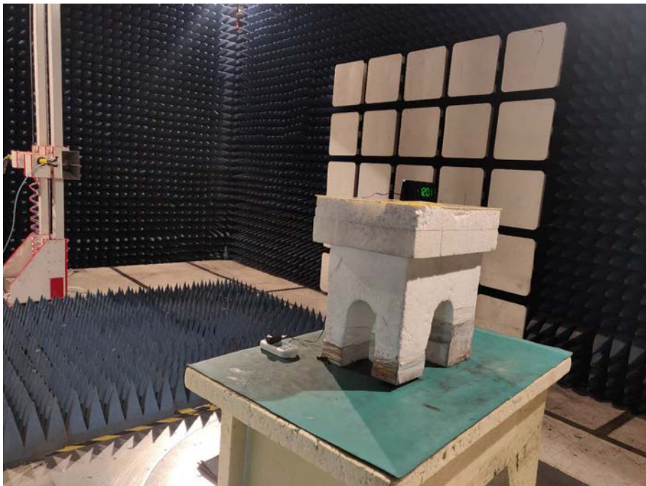
Spurious Emission Test Setup (Above 1GHz)
