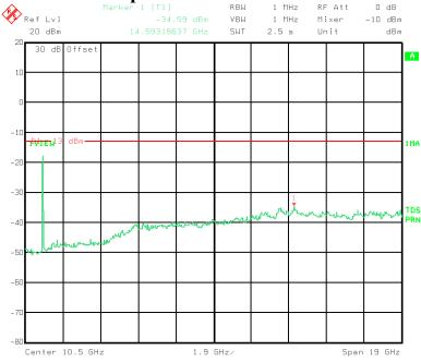
Title: 9L0482R LOW POWER MODULE W/VARIABLE BW MODULE-GSM-UPLINK Comment A: APSE06a.PCX Antenna Port Spurious Emissions (GSM)
