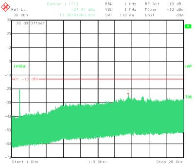
Title: 9L0482R LOW POWER MODULE W/VARIABLE BW MODULE-TDMA-UPLINK Comment A: APSE05a.PCX Antenna Port Spurious Emissions (NADC) Date: 18.NOV.1999 16:51:27
