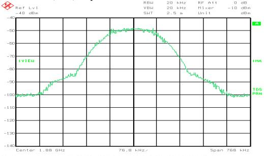
Title: 9L0482R LOW POWER MODULE W/VARIABLE BW MODULE-GSM-UPLINK Comment A: 0BW06b.PCX Occupied Bandwidth Input Signal (GSM) Channel 600 18.NOV.1999 19:52:58
