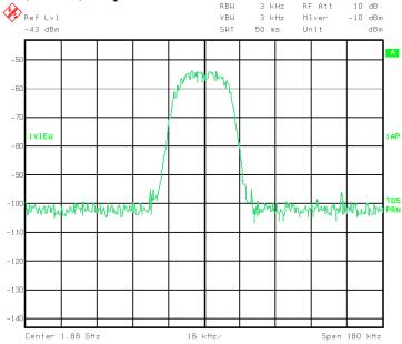
Title: 9L0482R LOW POWER MODULE W/VARIABLE BW MODULE-TDMA-UPLINK Comment A: OBW04b.PCX Occupied Bandwidth Input Signal (NADC) Date: 18.NOV.1999 16:19:35
