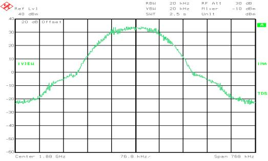
Title: 9L0482R LOW POWER MODULE W/VARIABLE BW MODULE-GSM-UPLINK Comment A: 0BW06a.PCX Occupied Bandwidth (GSM)
