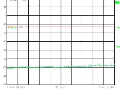
Title: 9L0482R LOW POWER MODULE W/VARIABLE BW MODULE-GSM-UPLINK Comment A: APSEO6b.PCX Antenna Port Spurious Emissions (GSM)
