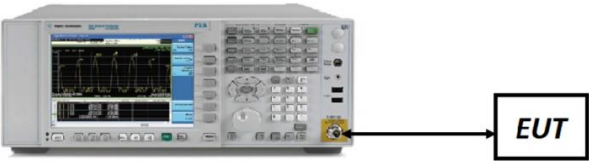
Figure 7-1. Test Instrument & Measurement Setup
