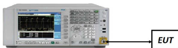
Figure 7-4. Test Instrument & Measurement Setup
