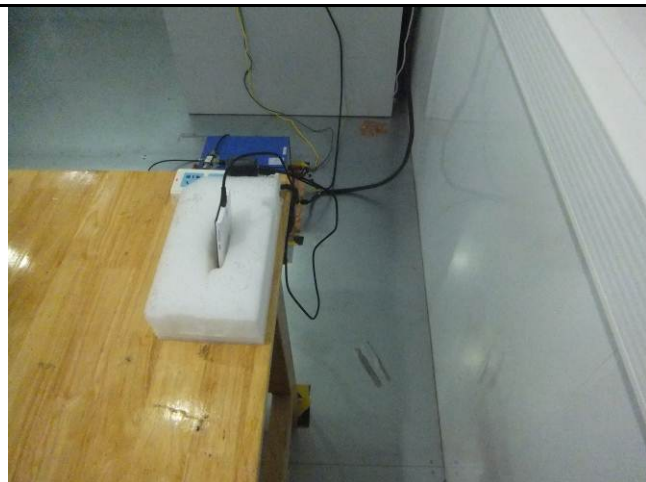
Conducted Emissions Test Setup Side View
