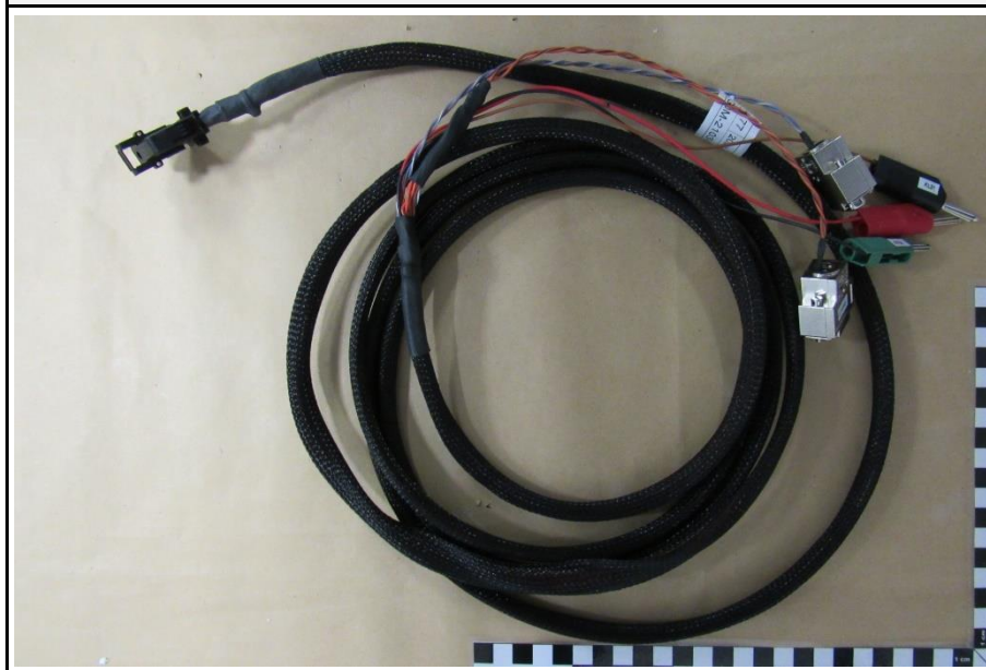
AE: Power and CAN cable
