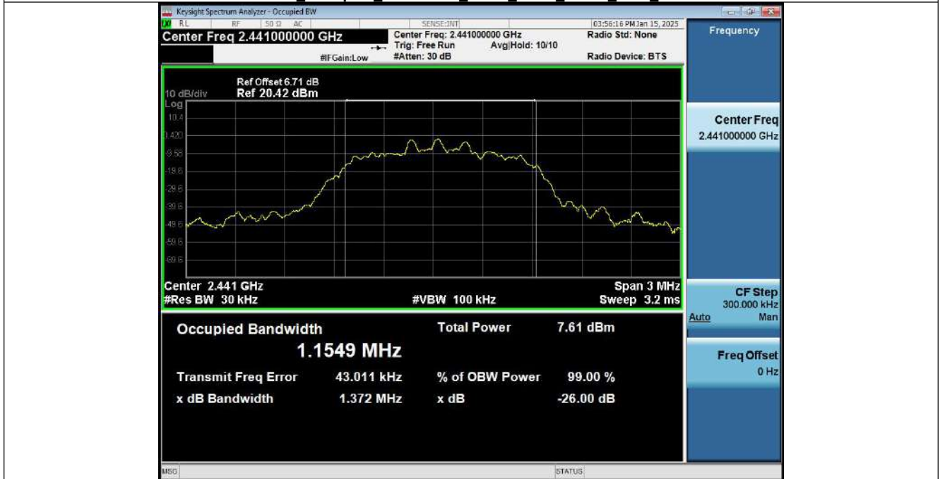
99% Occupied Bandwidth NVNT_ANT1_3-DH1_2441_00
