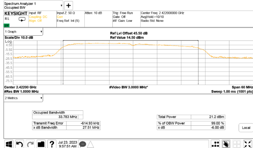
Plot 7.1.17 6 dB and 99% bandwidth test result at mid frequency
