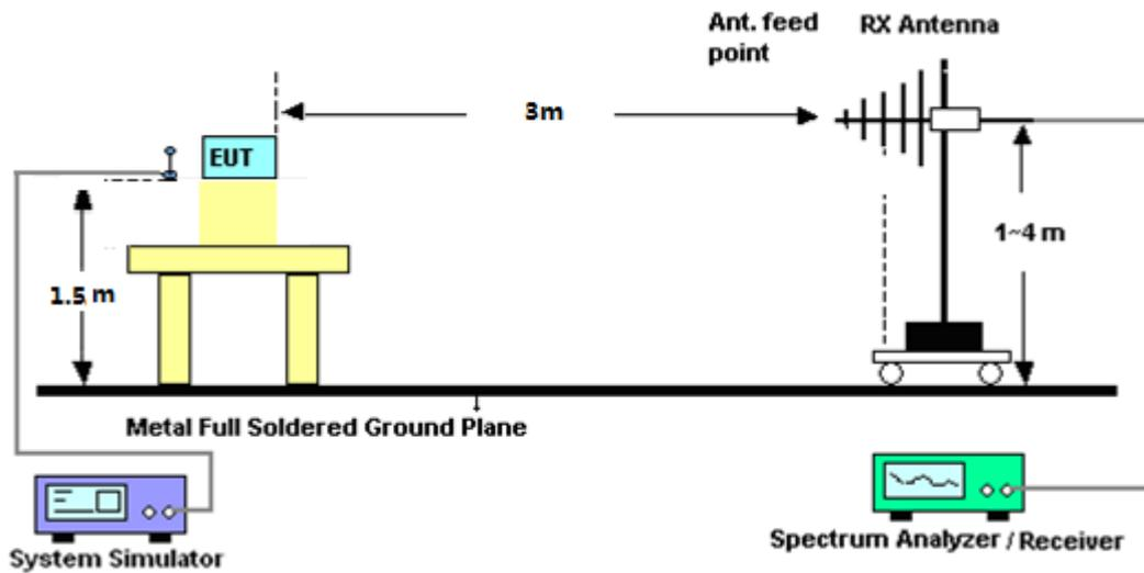
For radiated test from above 1GHz
