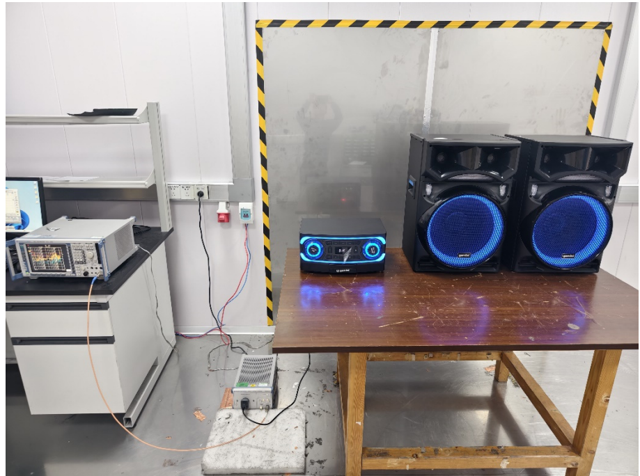
Conducted Emission Test Setup
