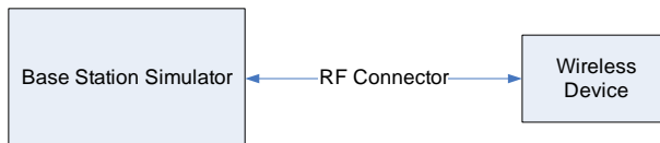
Figure 9-1 Power Measurement Setup
