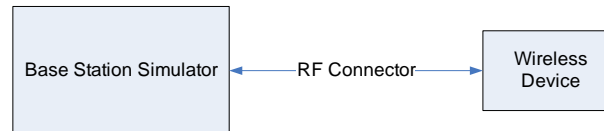
Figure 9-3 Power Measurement Setup
