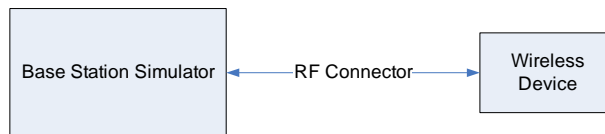
Figure 9-2 Power Measurement Setup
