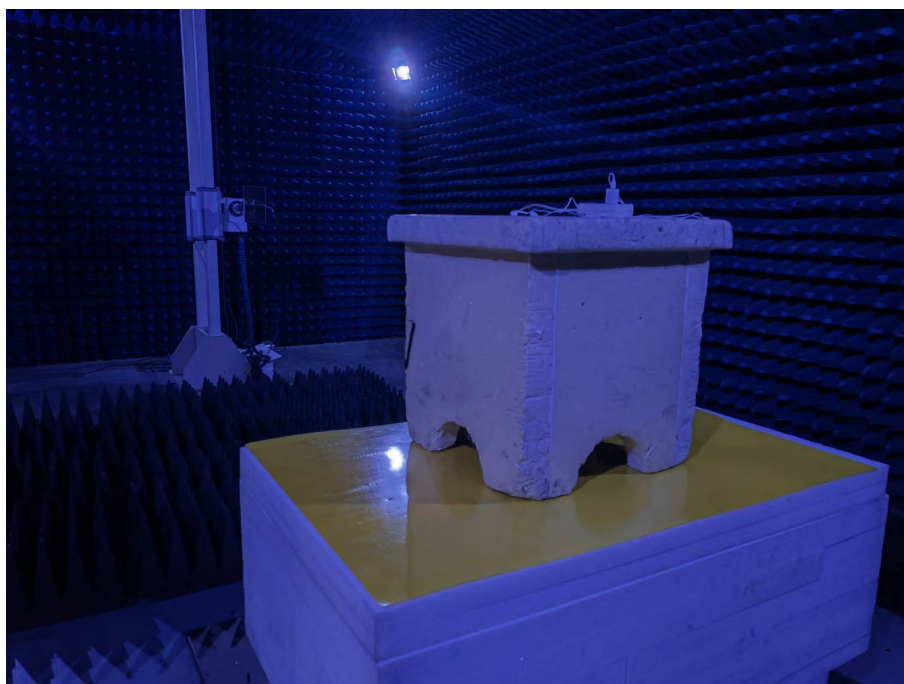
Photo of Radiated Emission Measurement (Above 1G)
