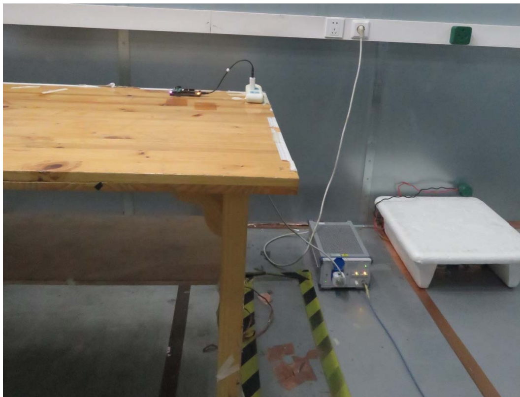
Picture 3 Conducted Emission Test Setup
