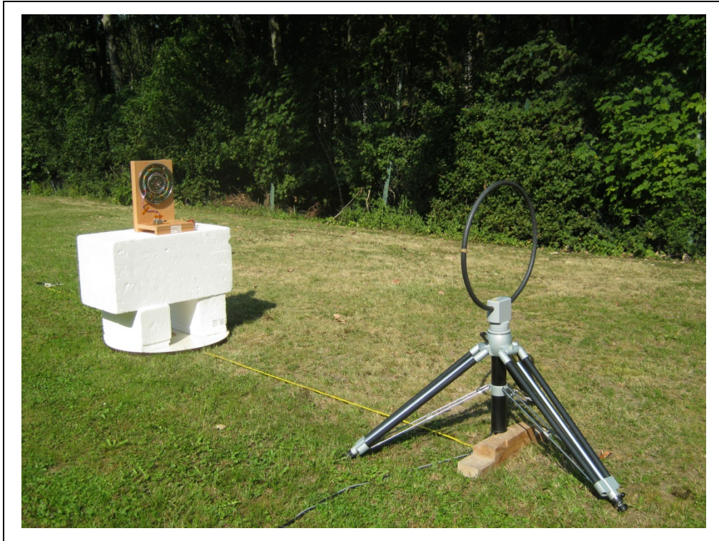
Photograph A1-3: Radiated emissions 9 kHz – 30 MHz at 3 m distance at open field site
