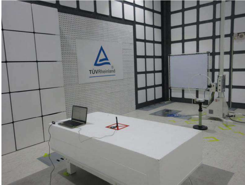
Photograph 5: Set-up for Spurious Emissions (Back View 3)
