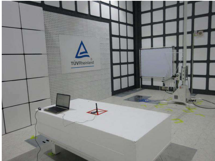
Photograph 3: Set-up for Spurious Emissions (Back View 1)
