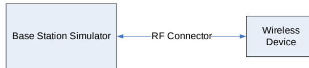
Figure 9-4 Power Measurement Setup
