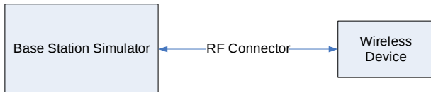
Figure 9-1 Power Measurement Setup
