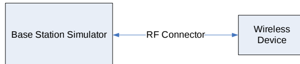
Figure 9-2 Power Measurement Setup
