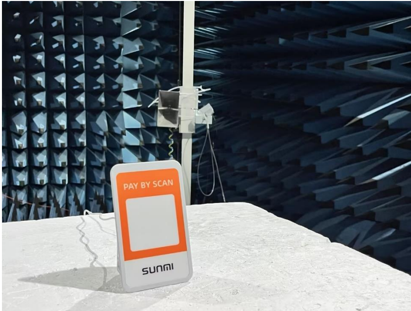
Radiated Spurious emissions test setup
