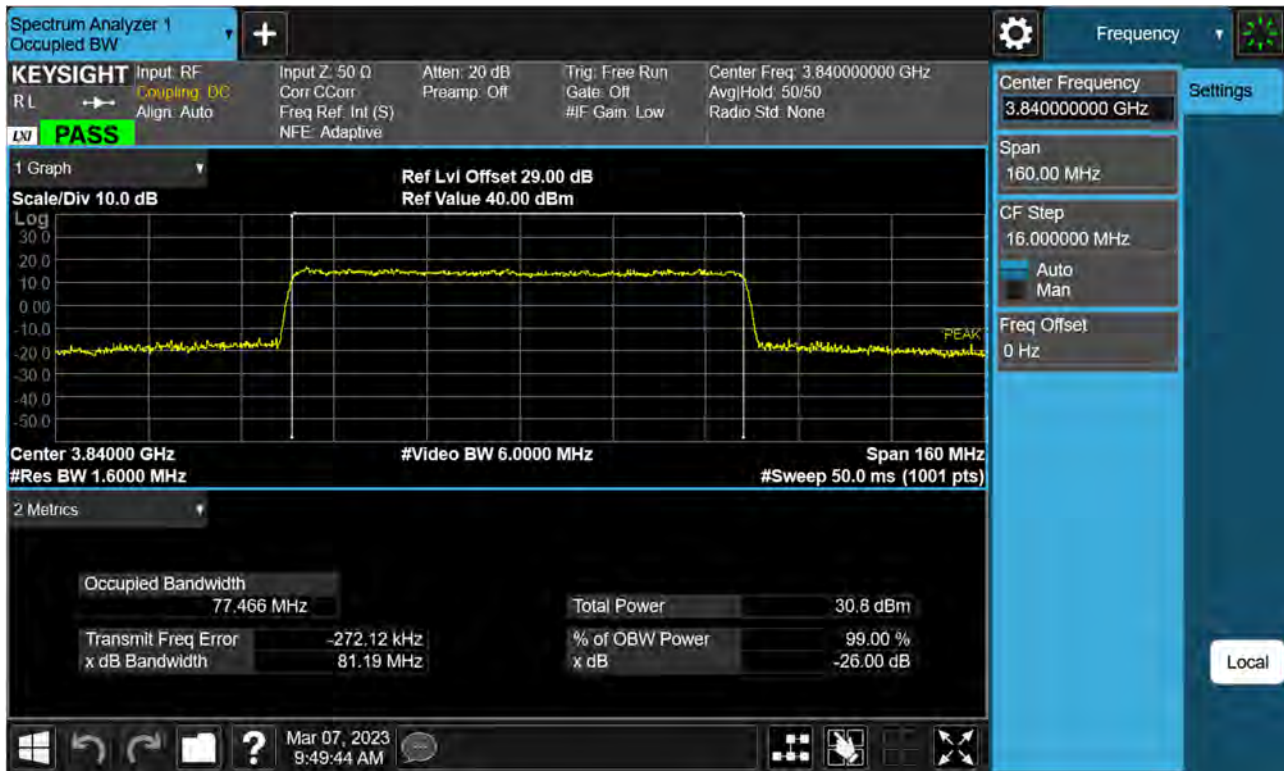
Sub6 n77(78). Occupied Bandwidth Plot (80 M BW Ch.656000 64QAM)
