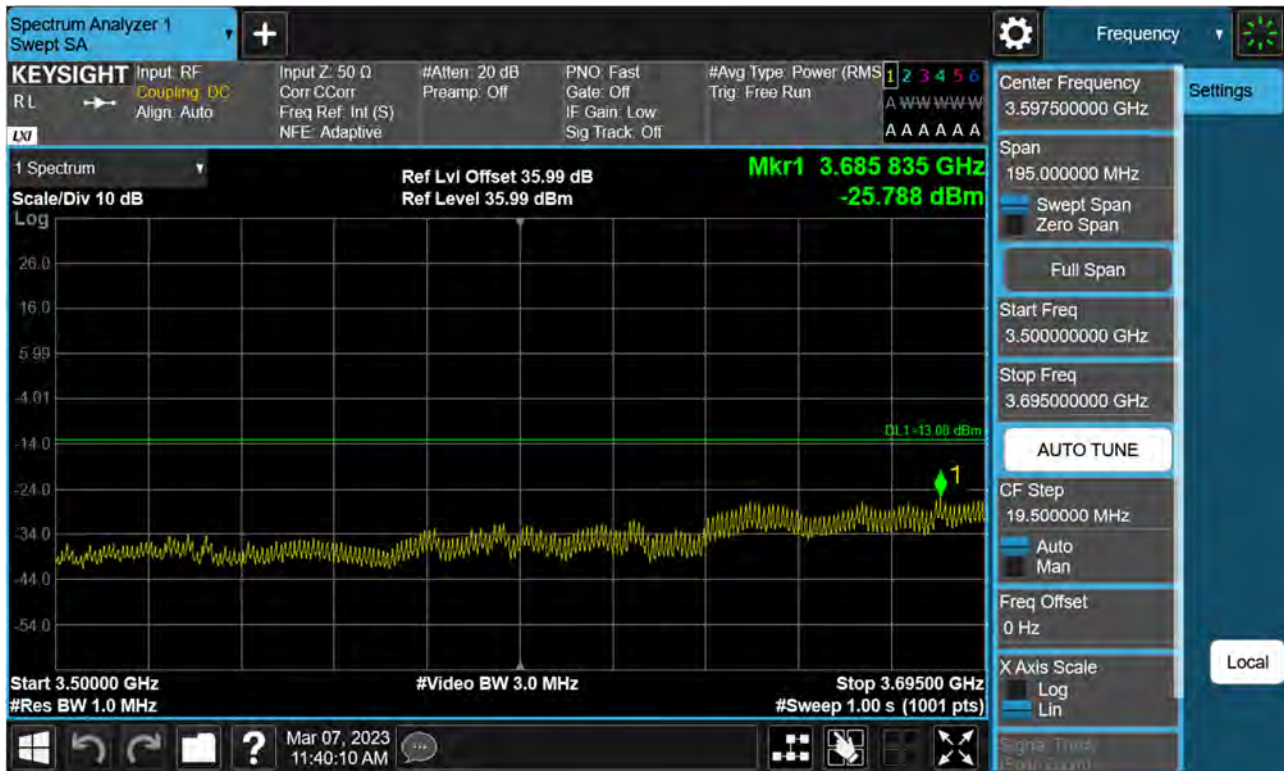
Sub6 n77(78). Low Band Edge Plot (70 M BW Ch.649000 BPSK FullIRB)(3)
