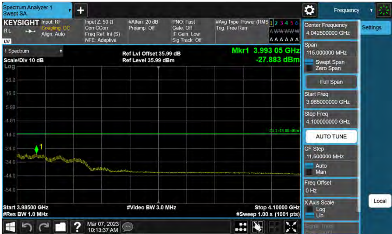
Sub6 n77(78). High Band Edge Plot (20 M BW Ch.664666 BPSK FullRB)(3)
