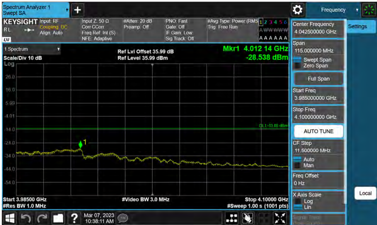
Sub6 n77(78). High Band Edge Plot (40 M BW Ch.664000 BPSK FullRB)(3)
