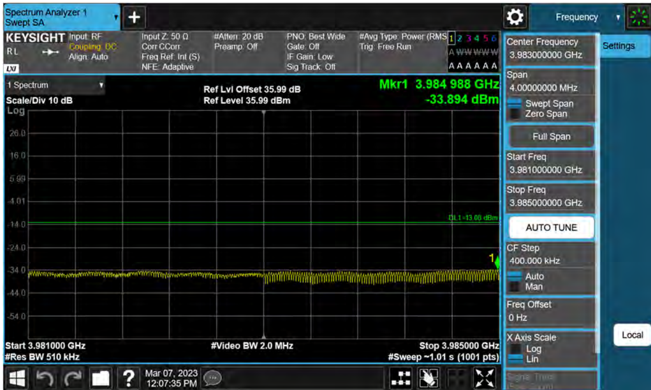
Sub6 n77(78). High Band Edge Plot (80 M BW Ch.662666 BPSK FullRB)(2)
