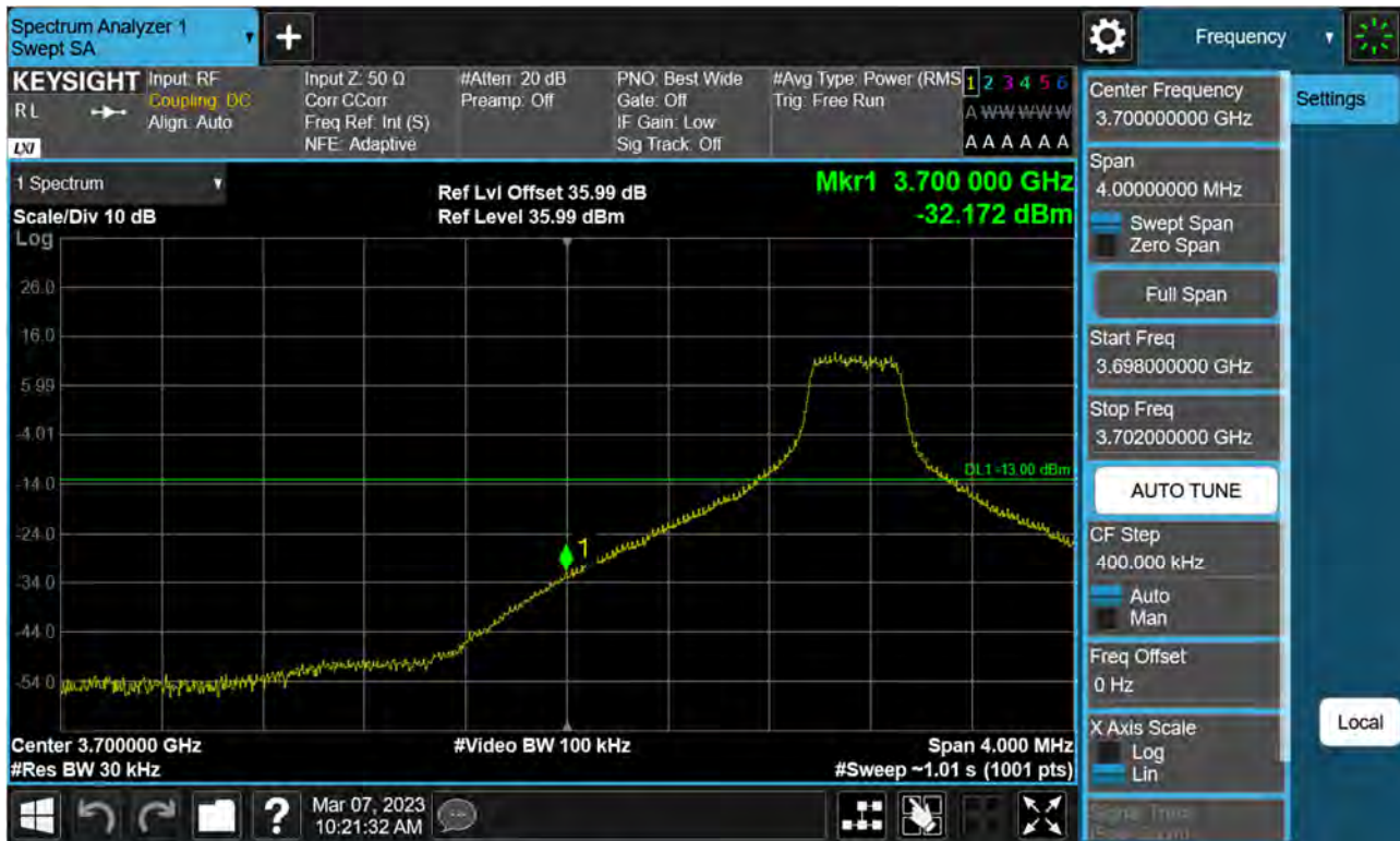
Sub6 n77(78). Low Band Edge Plot (30 M BW Ch.647668 BPSK 1RB)(1)
