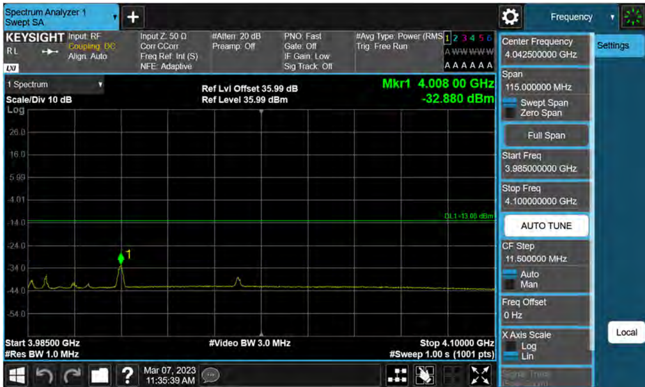
Sub6 n77(78). High Band Edge Plot (60 M BW Ch.663332 BPSK 1RB)(3)
