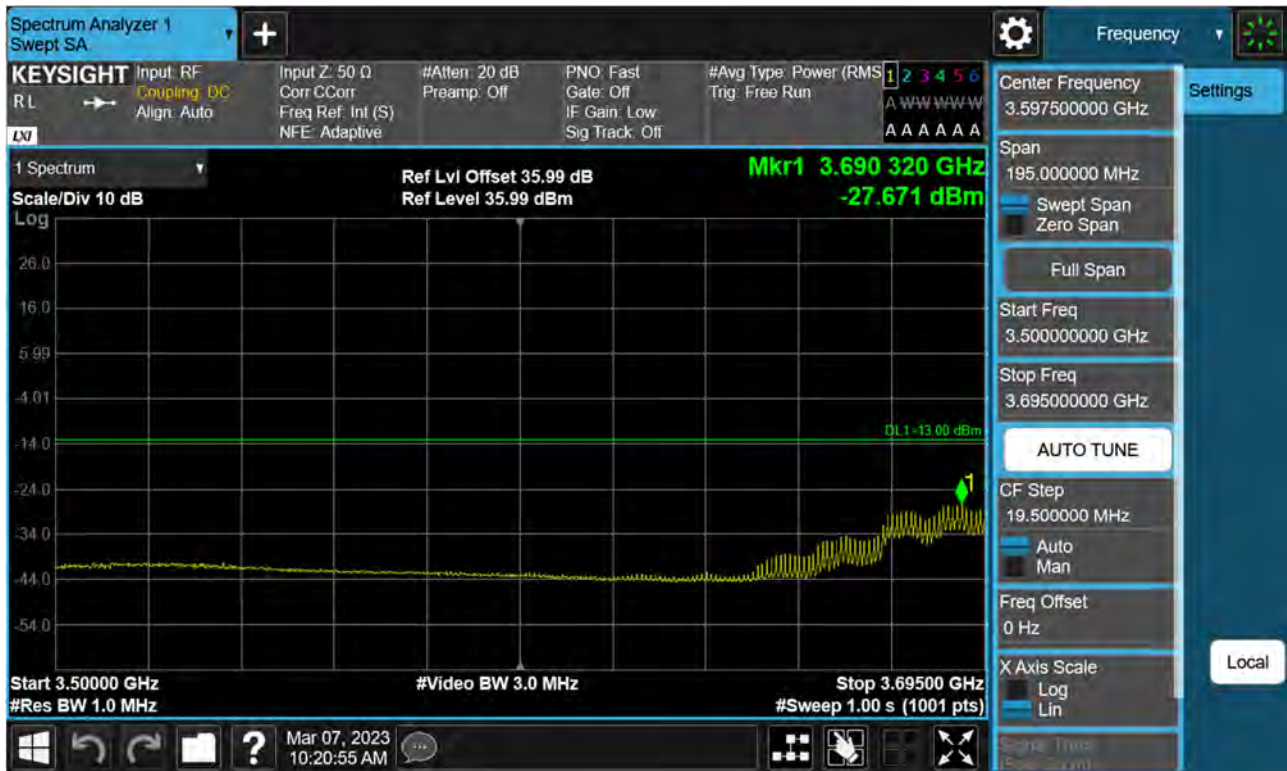
Sub6 n77(78). Low Band Edge Plot (30 M BW Ch.647668 BPSK FullIRB)(3)
