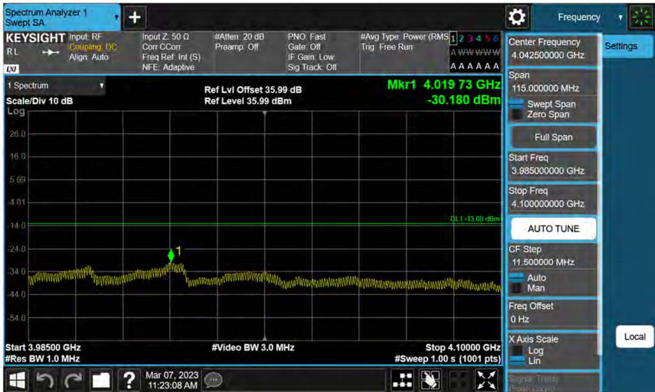
Sub6 n77(78). High Band Edge Plot (50 M BW Ch.663666 BPSK FullRB)(3)
