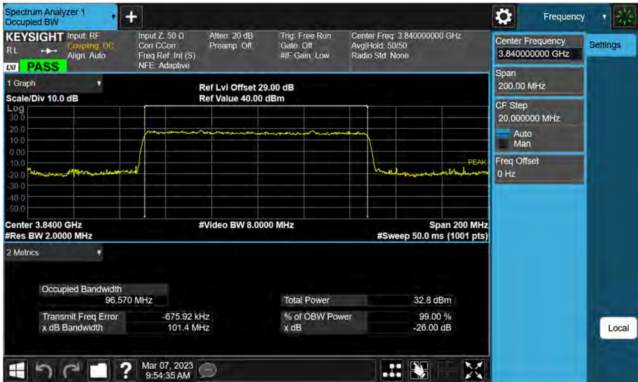
Sub6 n77(78). Occupied Bandwidth Plot (100 M BW Ch.656000 BPSK)
