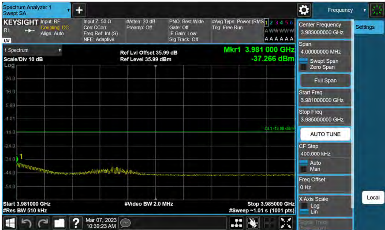
Sub6 n77(78). High Band Edge Plot (40 M BW Ch.664000 BPSK 1RB)(2)
