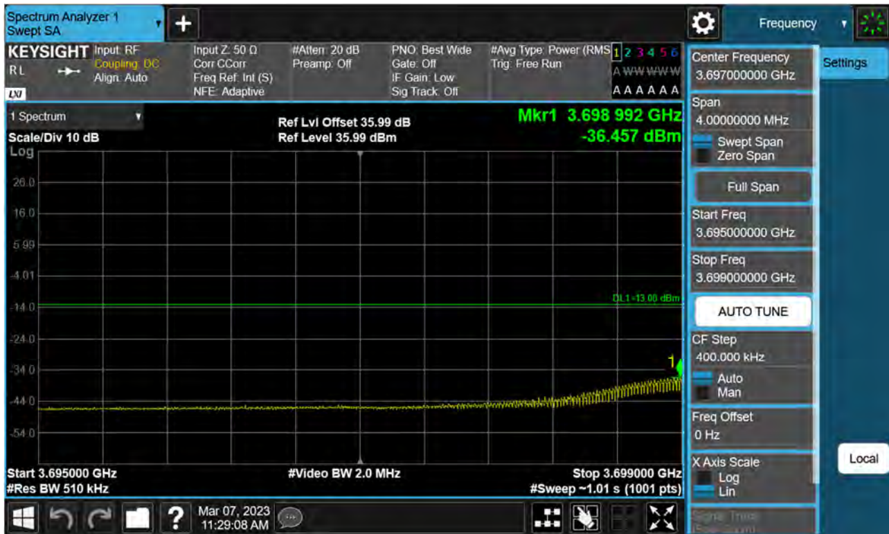
Sub6 n77(78). Low Band Edge Plot (60 M BW Ch.648668 BPSK 1RB)(2)
