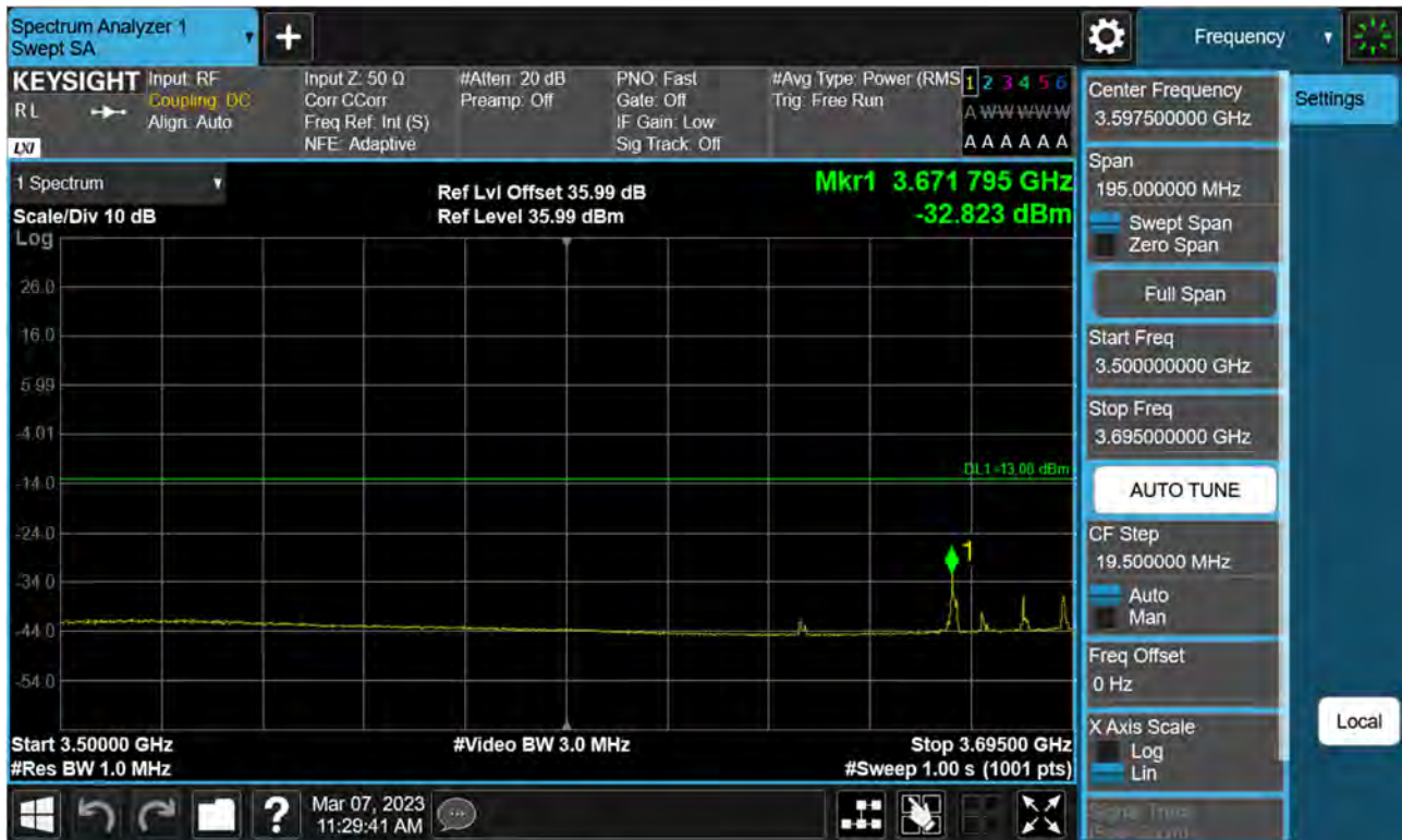
Sub6 n77(78). Low Band Edge Plot (60 M BW Ch.648668 BPSK 1RB)(3)
