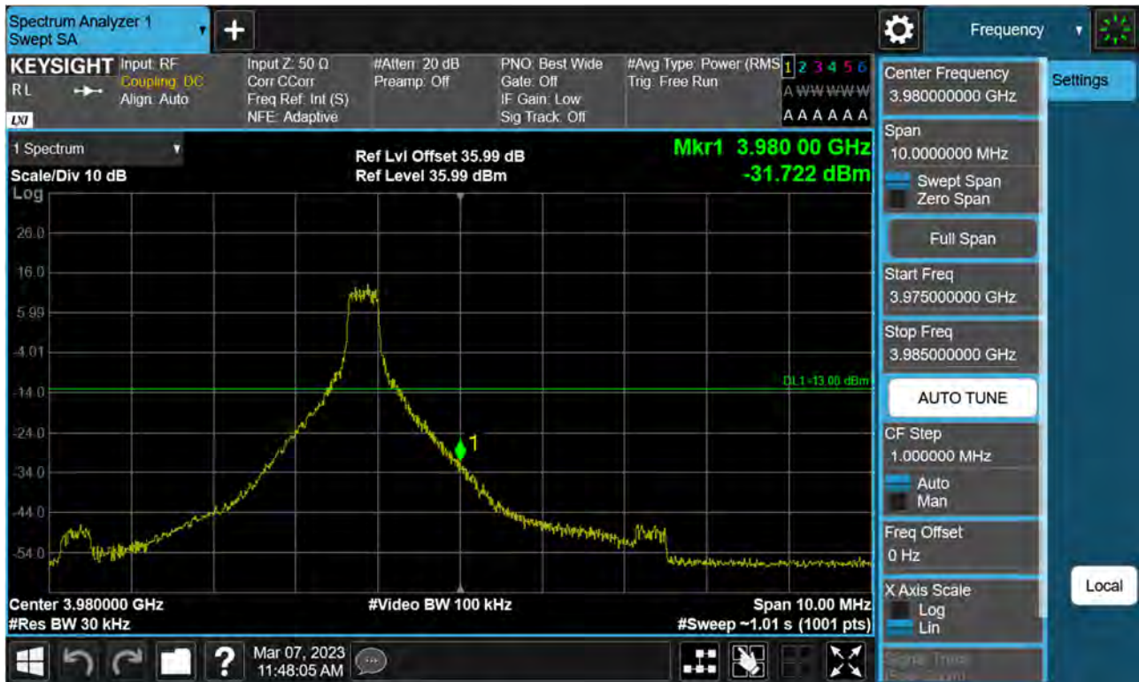
Sub6 n77(78). High Band Edge Plot (70 M BW Ch.663000 BPSK 1RB)(1)
