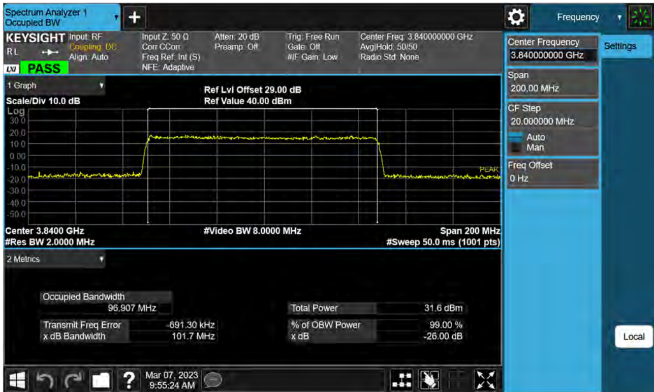
Sub6 n77(78). Occupied Bandwidth Plot (100 M BW Ch.656000 16QAM)
