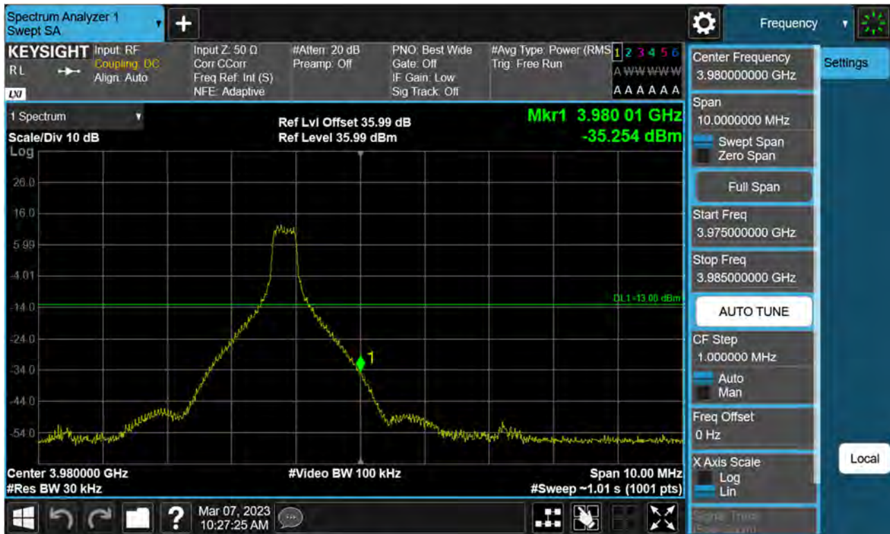
Sub6 n77(78). High Band Edge Plot (30 M BW Ch.664332 BPSK 1RB)(1)
