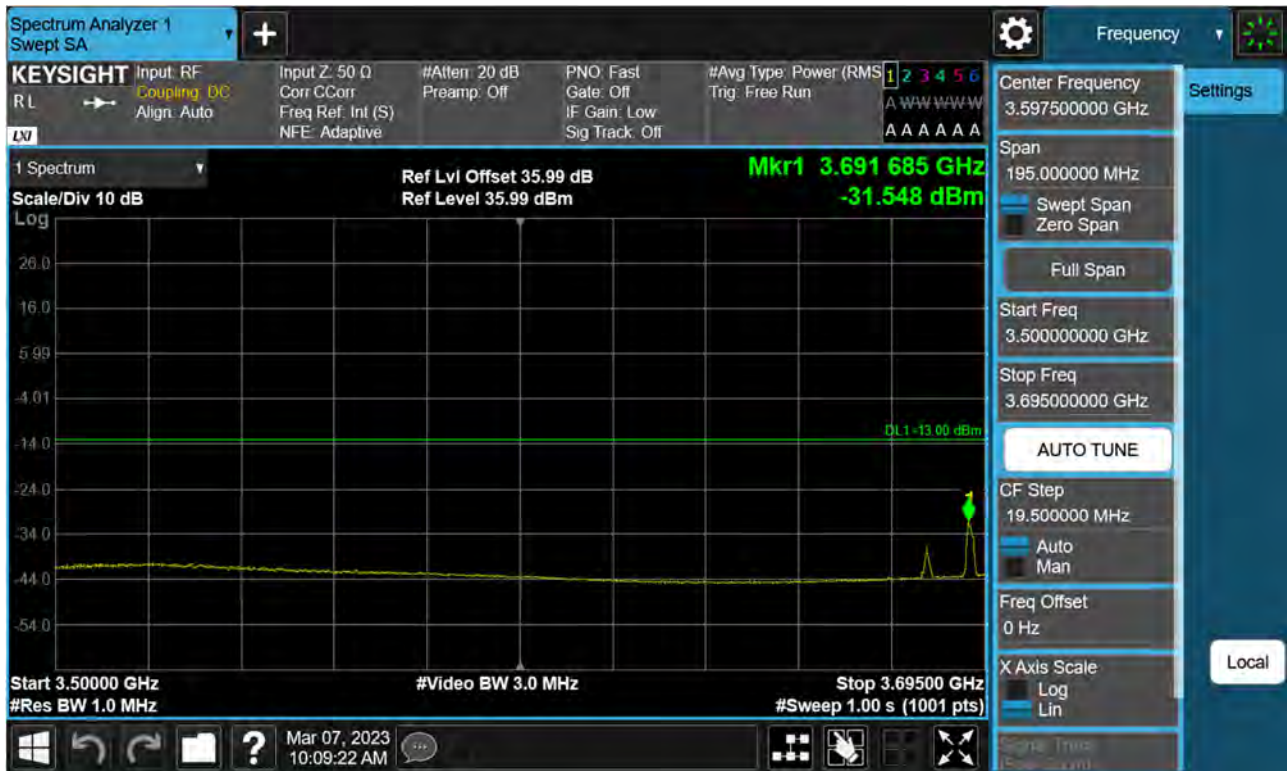
Sub6 n77(78). Low Band Edge Plot (20 M BW Ch.647334 BPSK 1RB)(3)
