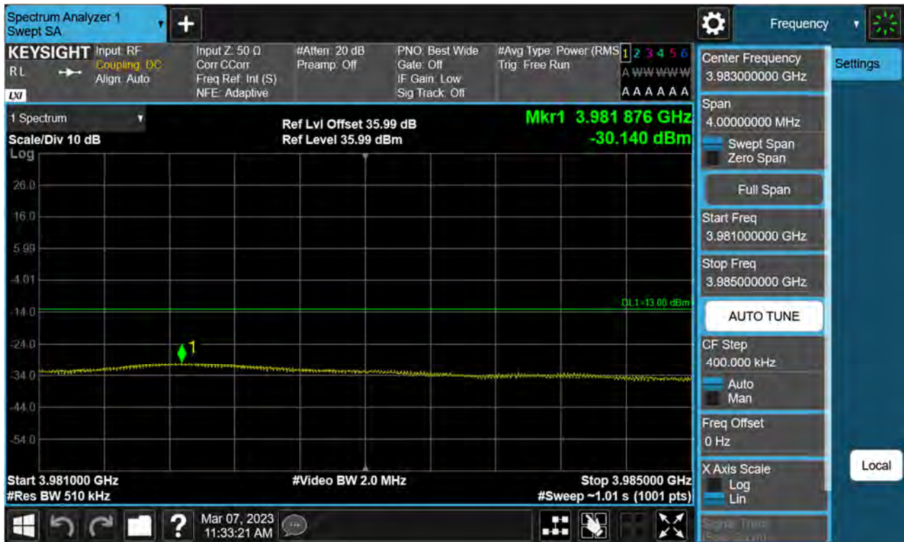
Sub6 n77(78). High Band Edge Plot (60 M BW Ch.663332 BPSK FullRB)(2)
