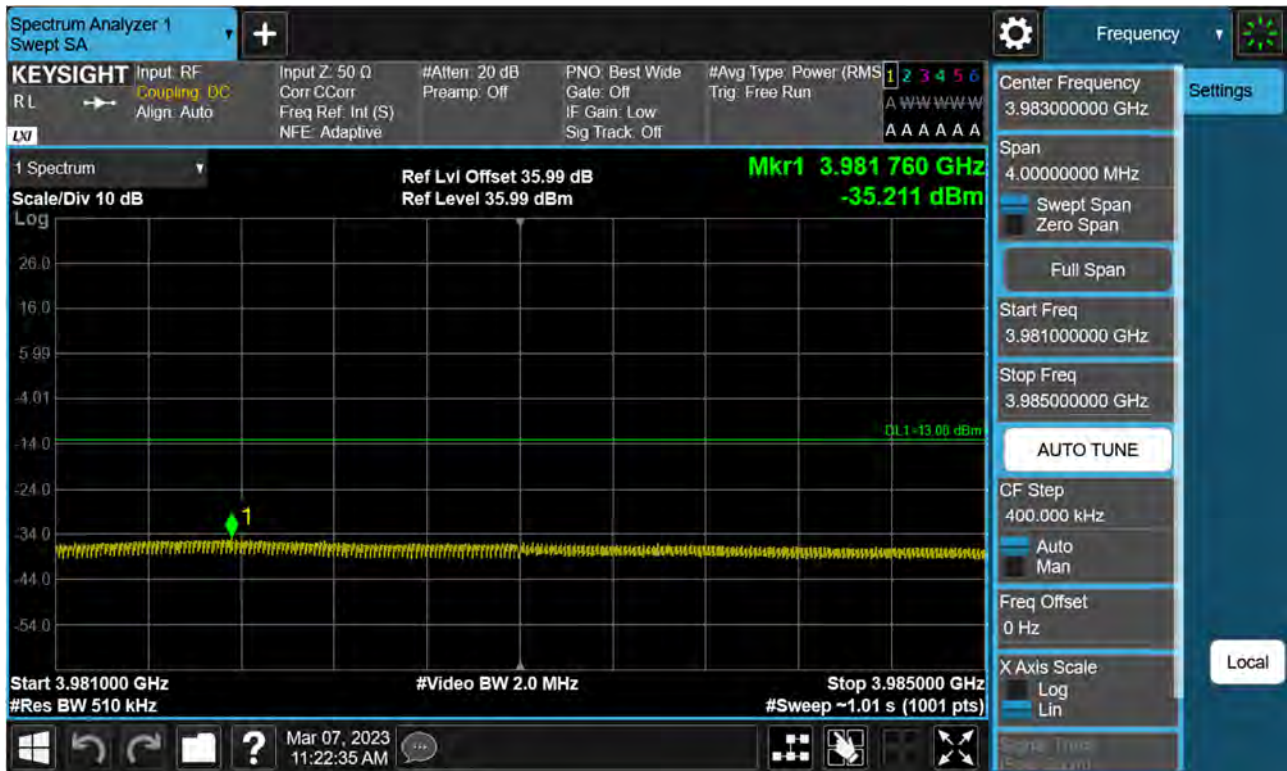
Sub6 n77(78). High Band Edge Plot (50 M BW Ch.663666 BPSK FullRB)(2)
