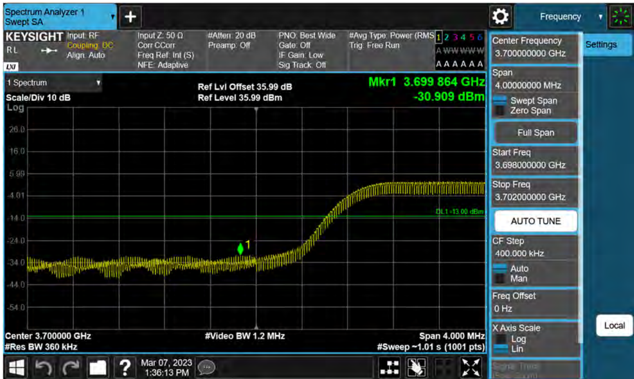
Sub6 n77(78). Low Band Edge Plot (90 M BW Ch.649668 BPSK FullRB)(1)
