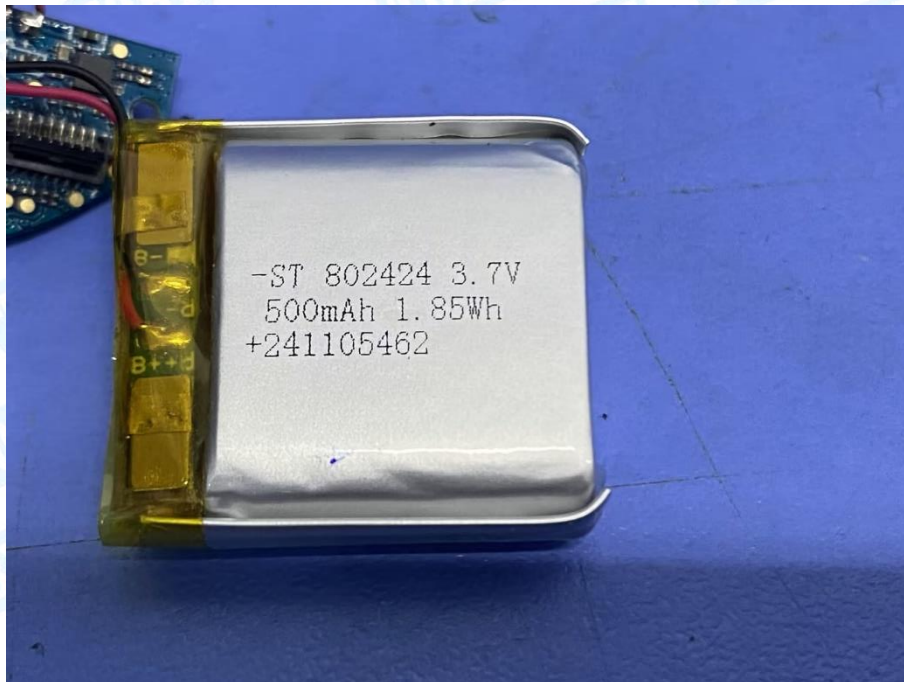
Photo 9 Internal of Battery
