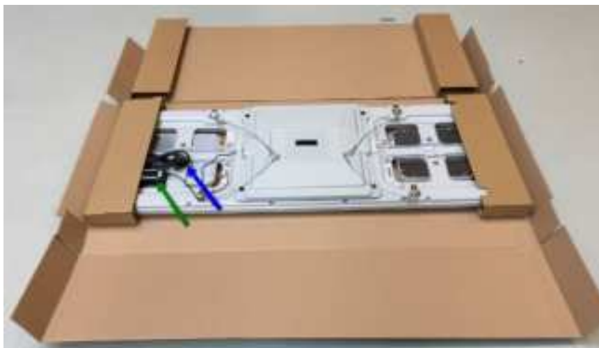
Figure 4. RTLS portal box content with powers supply (green arrow) and power cable (blue arrow).
