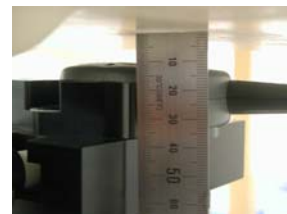
Figure 11. Mouth Face SAR Test Setup
