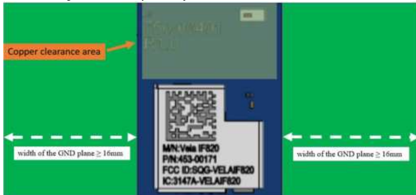
Figure 15: Integrated antenna variant layout suggestion example
