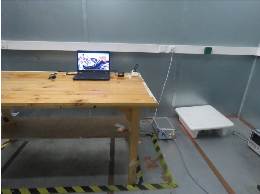
Conducted Emission Test Setup
