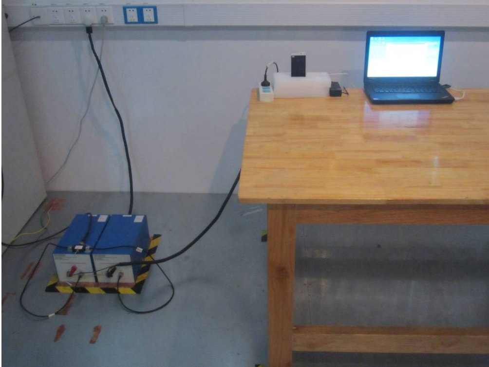
Conducted Emissions Test Setup Front View
