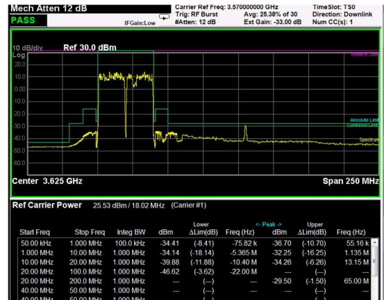
Low Band Edge, 2 Carrier, Modulation: QPSK, BW=20MHz
