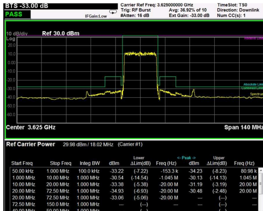
Middle Band Edge, 1 Carrier, Modulation: QPSK, BW=20MHz
