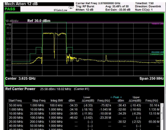
Low Band Edge, 2 Carrier, Modulation: 16QAM, BW=20MHz
