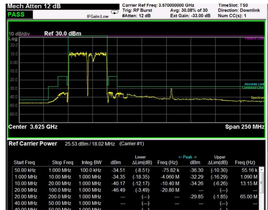
Low Band Edge, 2 Carrier, Modulation: 64QAM, BW=20MHz
