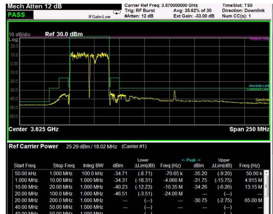
Low Band Edge, 2 Carrier, Modulation: 256QAM, BW=20MHz
