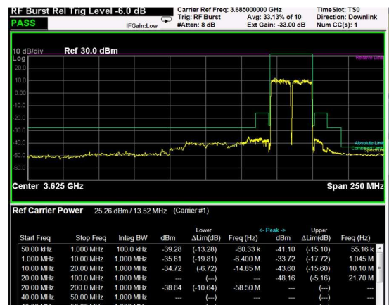
High Band Edge, 2 Carrier, Modulation: 256QAM, BW=15MHz
