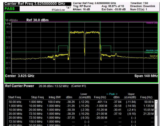
Middle Band Edge, 2 Carrier, Modulation: 256QAM, BW=15MHz
