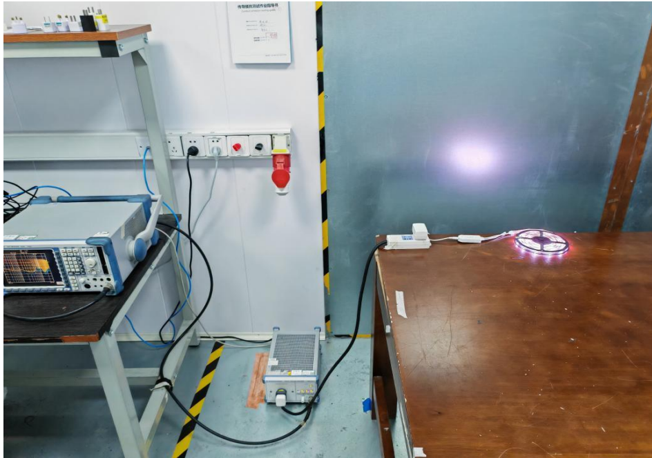
Conducted Emissions at Mains Terminals (150 kHz-30MHz)
