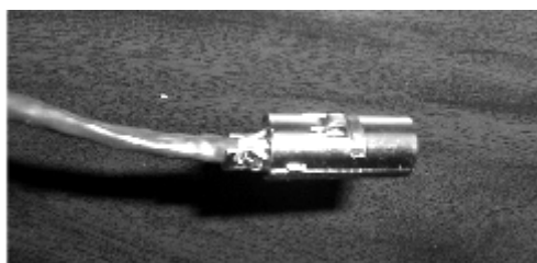
Figure 32. Metal Shell Placed Over 8-Pin DIN Connector
