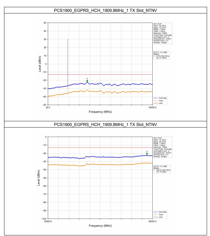
Note: All modes have been tested and we found GSM Test mode has the worst test result. Only record the worst test result.
