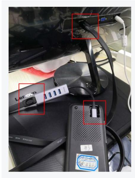
③After waiting for about 3-5 seconds, the display will display the image, then you can use the touchpad of the device;
