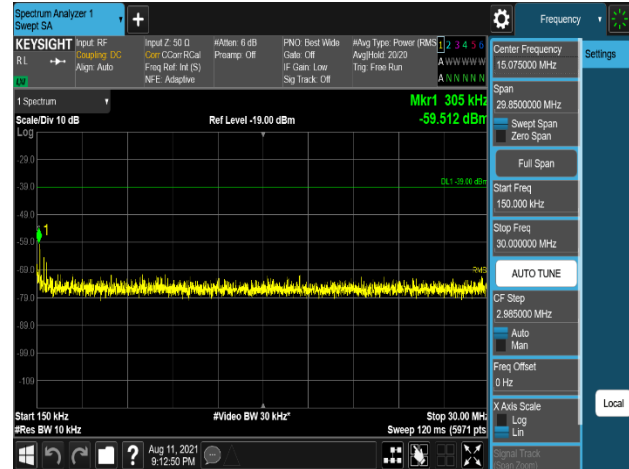
Plot 7-1082. Conducted Spurious Emission Plot 150 kHz to 30 MHz (B2_5M+5M+20M_3C_16QAM - Port 1)
