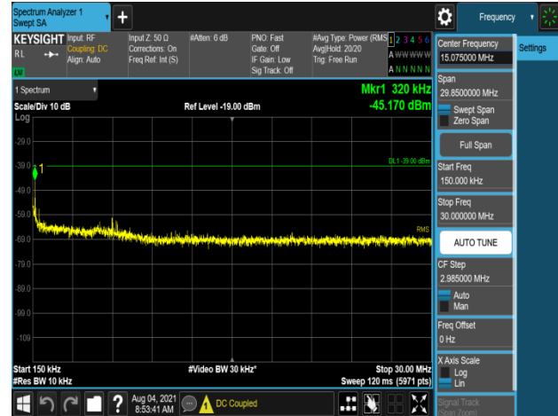
Plot 7-1112. Conducted Spurious Emission Plot 150 kHz to 30 MHz (B66_5M+5M_2C_16QAM - Mid Channel, Port 1)
