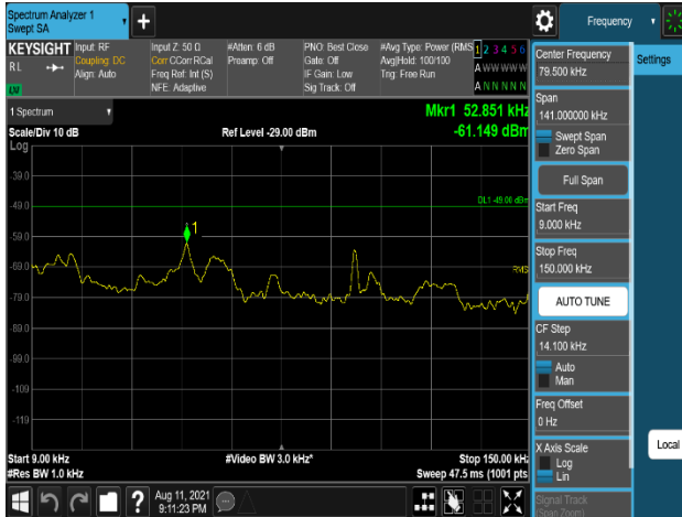
Plot 7-1081. Conducted Spurious Emission Plot 9 kHz to 150 kHz (B2_5M+5M+20M_3C_16QAM - Port 1)
