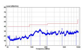
Site : chamber Condition: 3m HORIZONTAL Job No. : SZNS1211111-58026E-RF Test Mode: BTTransmitting
