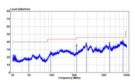
Site : chamber Condition: 3m HORIZONTAL Job No. : SZNS1211111-58026E-RF Test Mode: BTTransmitting
