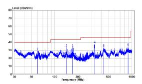
Site : chamber Condition: 3m VERTICAL Job No. : SZNS1211111-58026E-RF Test Mode: BTTransmitting
