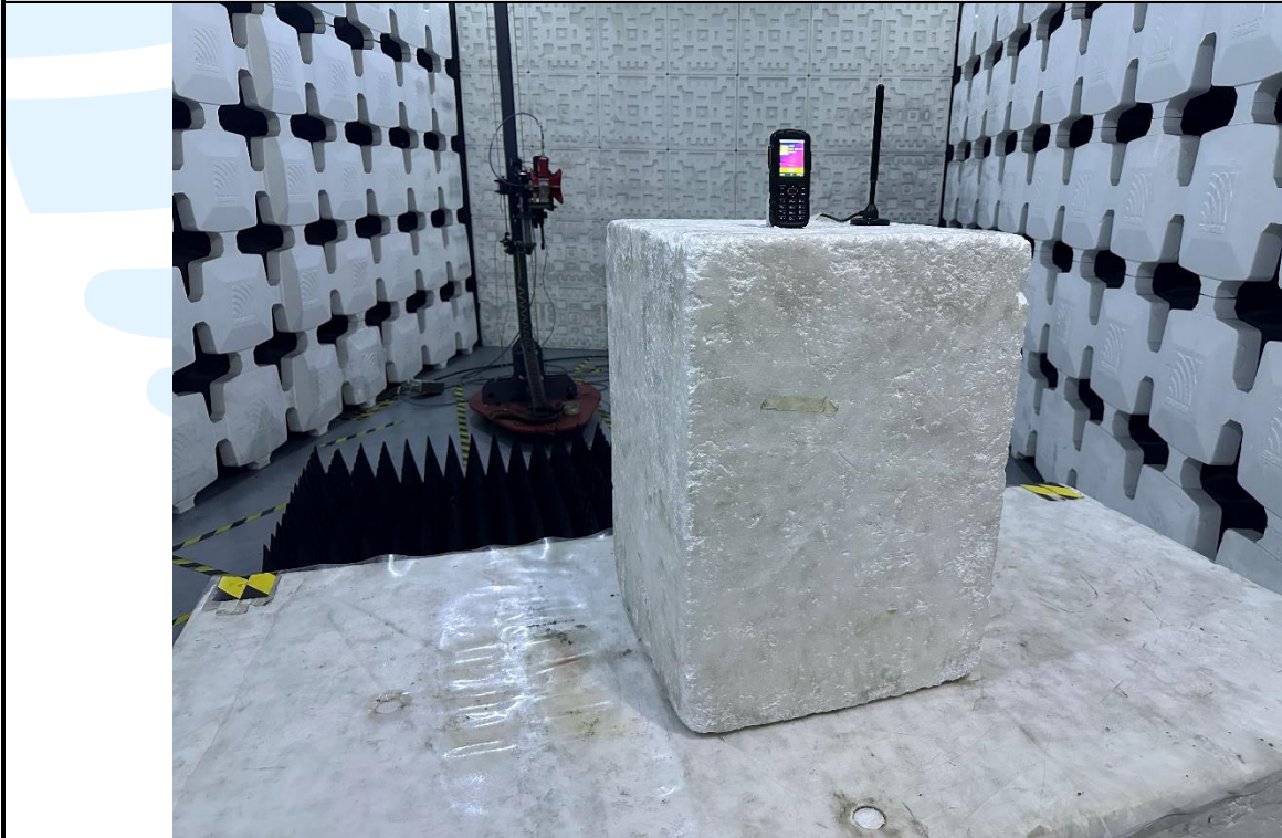
Radiated emission Test Setup (Above 1 GHz)
