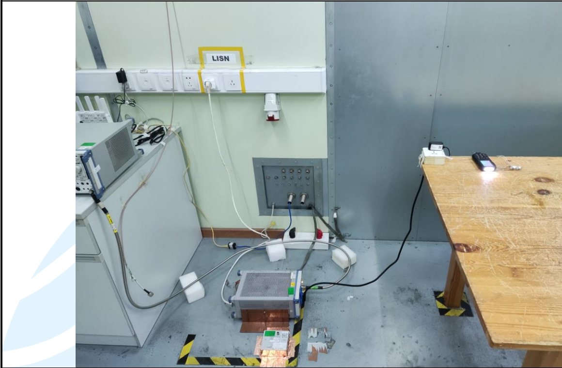
Conducted Emission Test Setup
