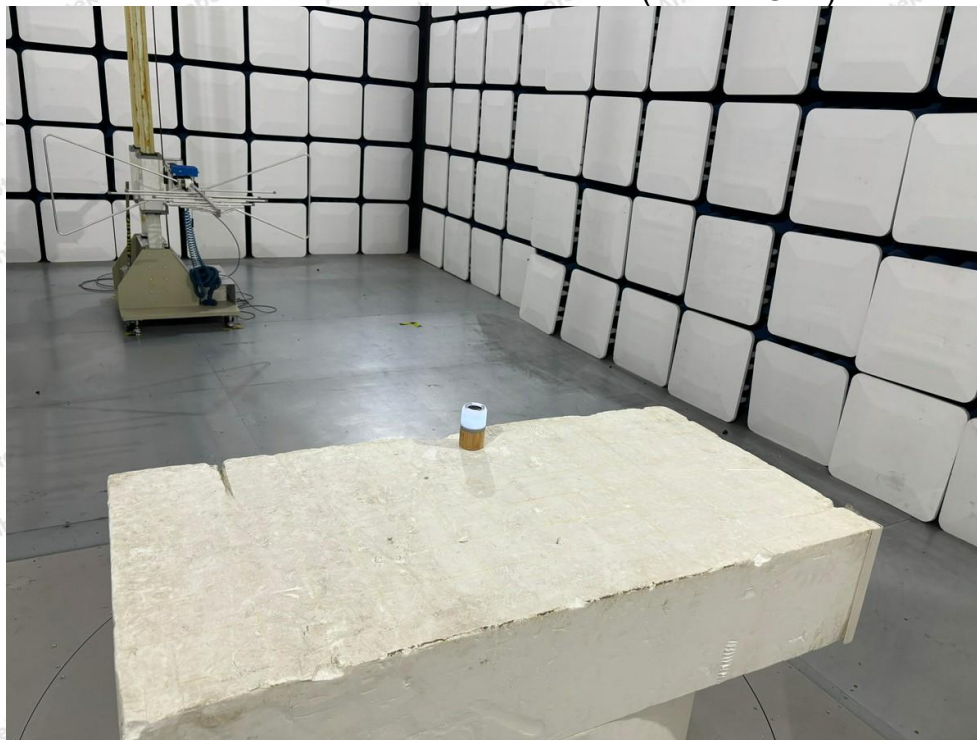
Photo of Radiation Emission Test (below 1GHz)
