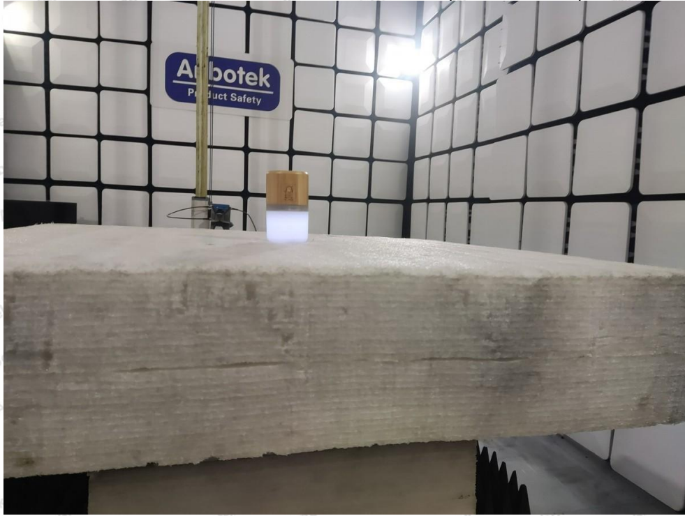
Photo of Radiation Emission Test (above 1GHz)
