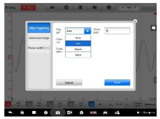
Figure 9-55 Sample Trigger Mode Screen
