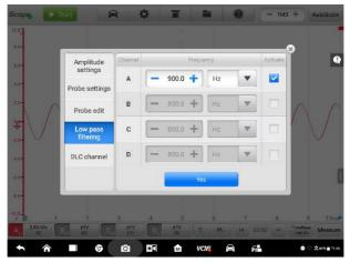
Figure 9-47 Sample Lowpass Filtering Screen
