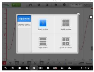
Figure 9-22 Sample Display Mode Selection Screen
