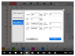
Figure 9-59 Sample Pulse Width Settings Screen
