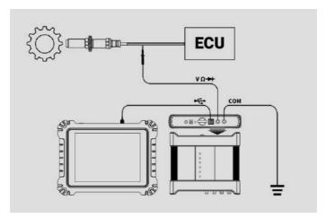
Figure 9-13 Sample Pulse Waveform Connection Diagram
