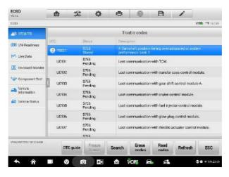
Figure 4-30 Sample DTC & FFD Screen
