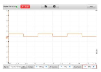
Figure 9-24 Sample Duty Cycle Setting Screen 1
