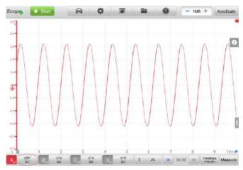
Figure 9-38 Sample Amplitude Setting Screen (DC 5V)
