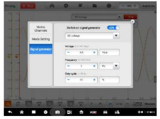
Figure 9-16 Sample Signal Generator Settings Screen
