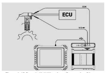
Figure 9-15 Sample X+Y Waveform Connection Diagram
