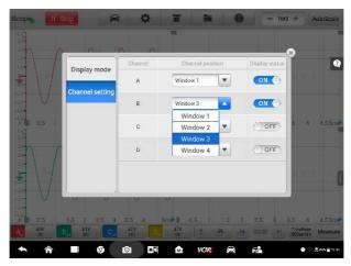
Figure 9-23 Sample Channel Setting Screen
