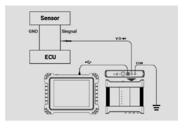
Figure 9-1 Sample Connection Diagram
