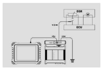
Figure 9-11 Sample DC Voltage Connection Diagram
