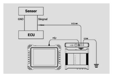
Figure 9-16 Sample Triangle Waveform Connection Diagram
