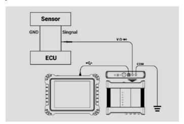
Figure 9-17 Sample Arbitrary Waveform Connection Diagram
