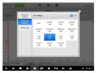
Figure 9-16 Sample Amplitude Setting Screen (AC 2.0V/div)
