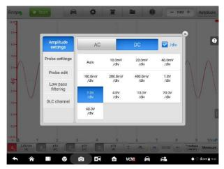
Figure 9-39 Sample Amplitude Setting Screen (AC 2.0V/div)
