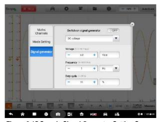
Figure 9-15 Sample Signal Generator Setting Screen
