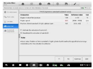
Figure 4-23 Sample Active Test Screen
