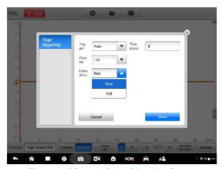
Figure 9-25 Sample Pulse Direction Screen
