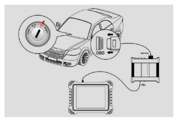
Figure 9-1 Sample Connection Diagram
