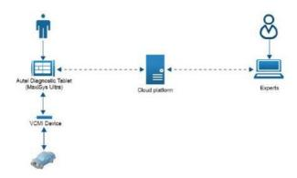
Figure 7-1 Principles of Remote Programming
