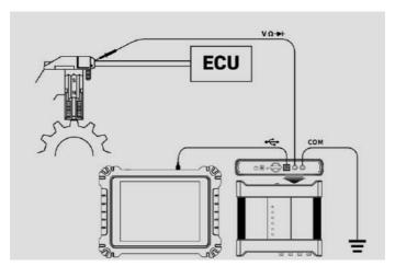
Figure 9-14 Sample Sinusoid Connection Diagram
