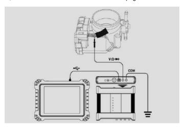
Figure 9-1 Sample Connection Diagram
