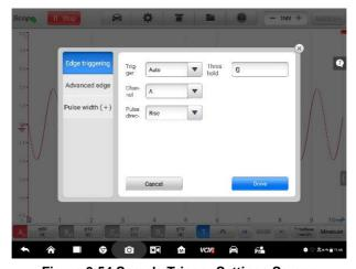
Figure 9-54 Sample Trigger Settings Screen
